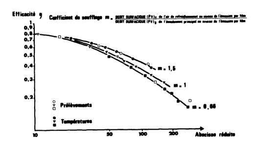
Blowing coefficient, m =  $\frac{\text{surface flow rate (pV)}_{c} \text{ of cooling air at the point }}{\text{surface flow rate (pV)}_{g}} \text{ of main flow at the point }}{\text{of film emission}}$
