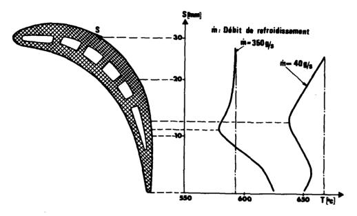
$\frac{\text{Key}\colon}{\mathring{\textbf{m}}\colon \text{ D\'ebit de refroidissement = cooling flow rate, }\mathring{\textbf{m}}$
