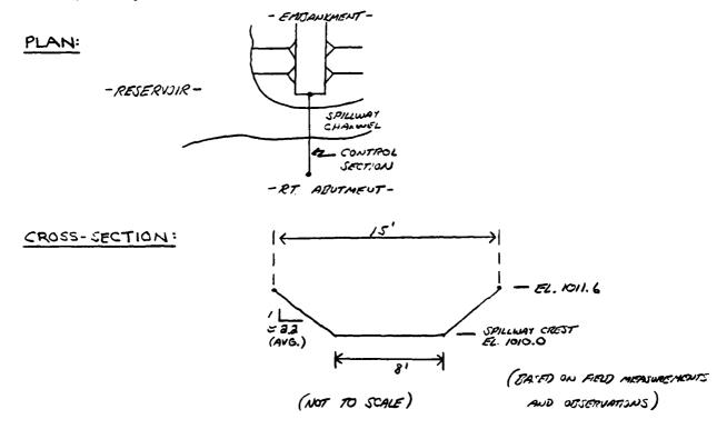
THE SPILLIAY RATING TROLE IS PROVIDED ON SHEET 20, ALD IS SASED ON THE ASSUMPTION OF CRITICAL DEPTH AT THE CONTROL SECTION, WITH NO APPROACH LOSSES (SEE SMEETS ZAND 8 FOR ASSUMPTIONS AND METHODOLOGY).
