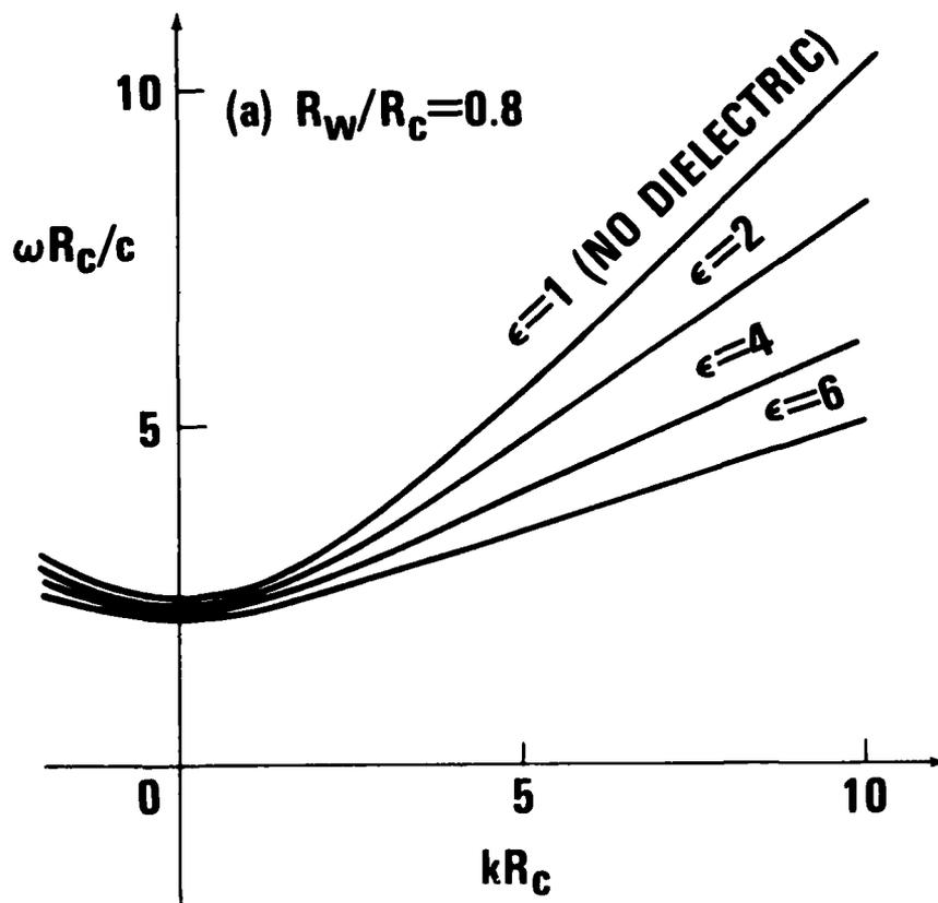
FIGURE 11a PLOT OF THE VACUUM TM MODE DISPERSION RELATION IN THE PARAMETER SPACE  $(\omega, k)$  OBTAINED FROM EQS. (48), (50), AND (51) FOR  $R_w/R_c = 0.8$  AND SEVERAL VALUES OF THE DIELECTRIC CONSTANT  $\epsilon$ .
