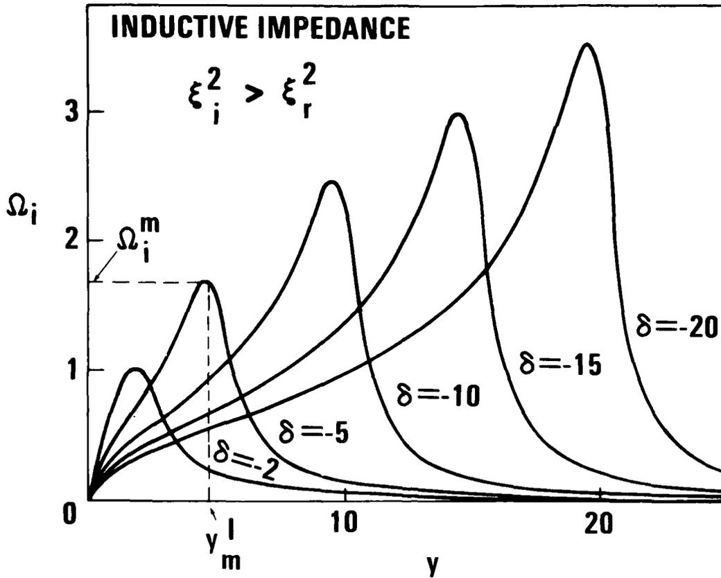
FIGURE 2 PLOT OF THE NORMALIZED GROWTH RATE  $\Omega_i$  VERSUS  $y$  [EQ. (27)] FOR  $\xi_i^2 > \xi_r^2$  AND SEVERAL VALUES OF  $\delta$ .
