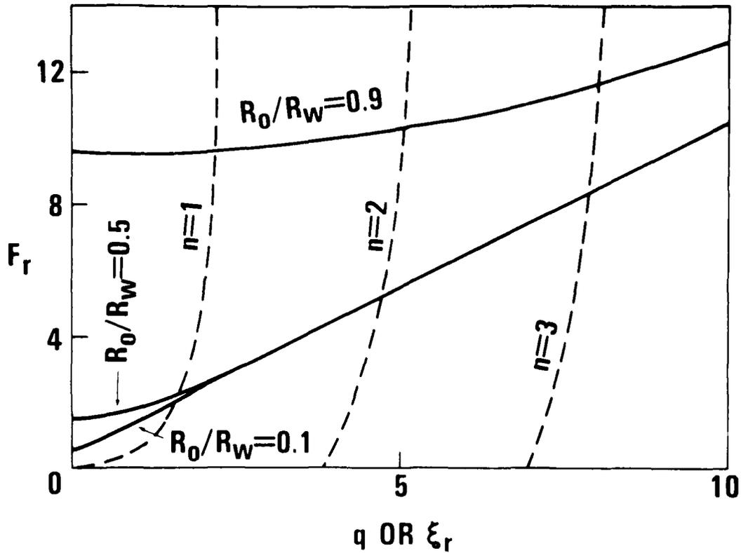
FIGURE 6 PLOT OF THE ADMITTANCE  $F = F_r$  VERSUS  $\xi = \xi_r$  (DASHED CURVES) OBTAINED FROM EQ. (18) AND  $F_r$  VERSUS  $q$  (SOLID CURVES) OBTAINED FROM EQ. (38) FOR  $R_0/R_w = 0.1, 0.5, \text{ AND } 0.9$ . THE HORIZONTAL SCALE REPRESENTS BOTH  $\xi_r$  AND  $q$ .
