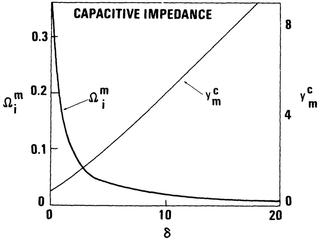
FIGURE 5 PLOT OF THE NORMALIZED MAXIMUM GROWTH RATE  $\Omega_i^m$  AND CORRESPONDING  $y_m^c$  VERSUS  $\delta$  [EQ. (27)] FOR  $\xi_r^2 > \xi_i^2$ .
