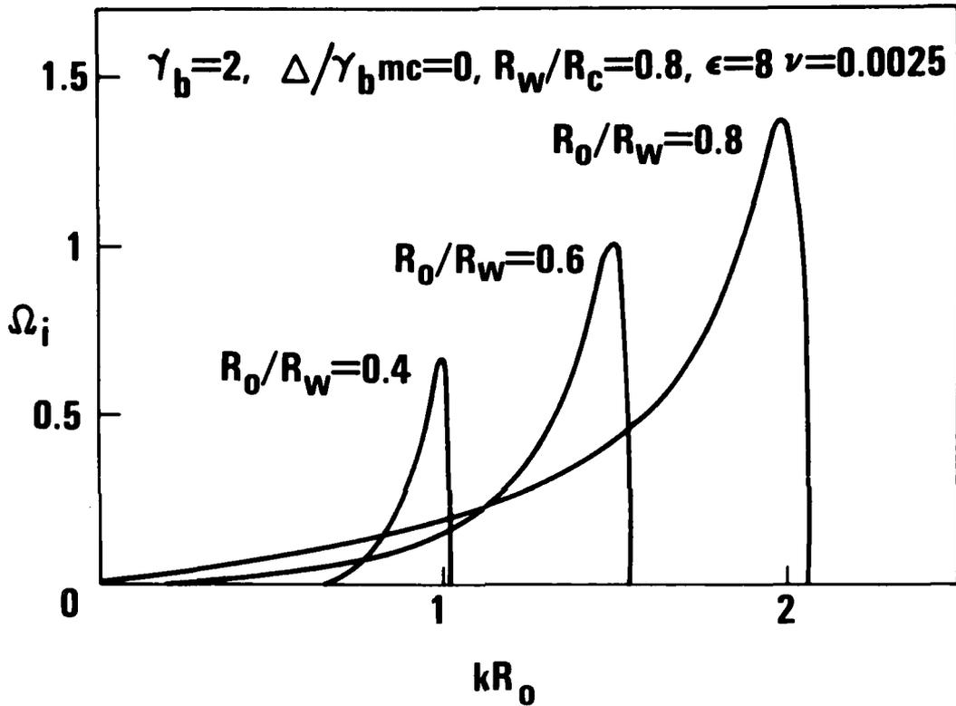
FIGURE 14 PLOT OF THE NORMALIZED GROWTH RATE  $\Omega_i = 1m\Omega$  VERSUS  $kR_0$  [EQ. (61)]
