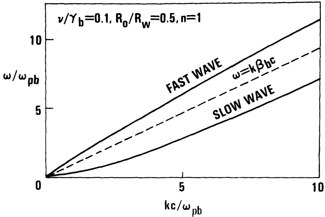
**FIGURE 9** PLOT OF THE DISPERSION CURVE IN THE PARAMETER SPACE  $(\omega, k)$  FOR  $n = 1, R_0/R_w = 0.5, \gamma_b = 3,$  AND  $v/\gamma_b = 0.1.$  THE DASHED STRAIGHT LINE  $\omega = k\beta_{bc}$  IS THE FREE-STREAMING MODE.
