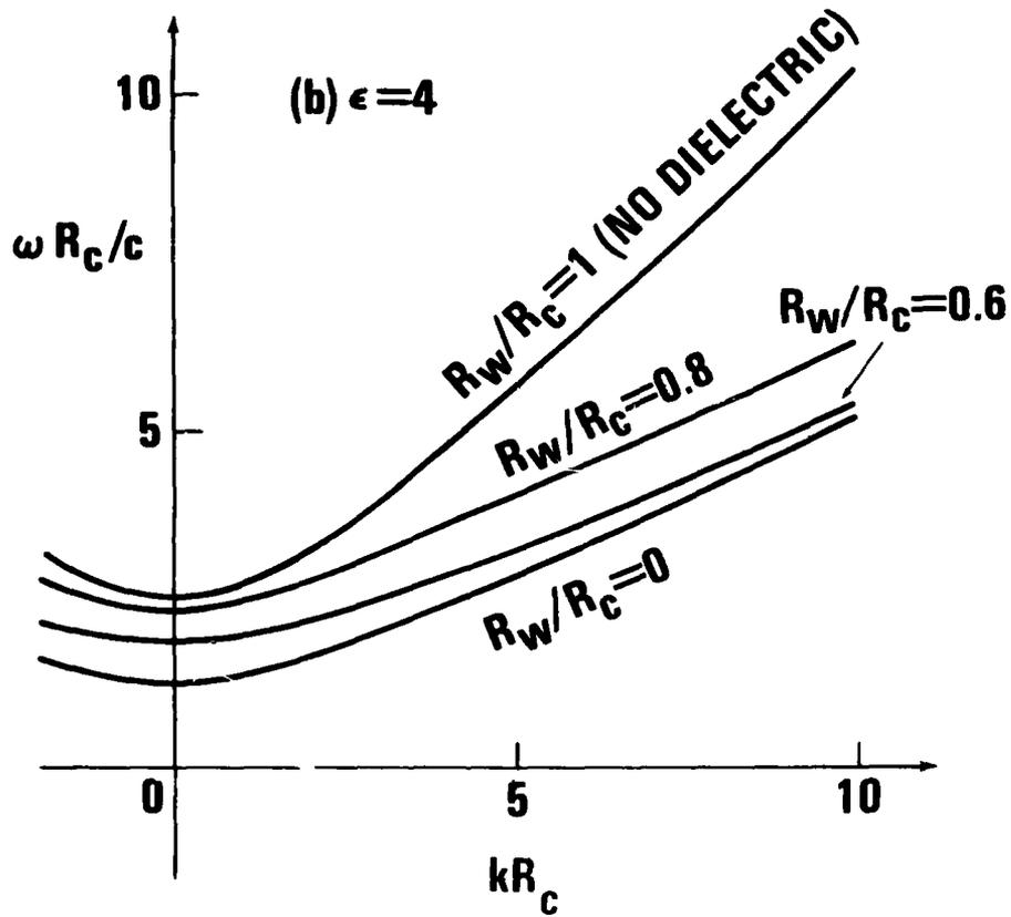
FIGURE 11b PLOT OF THE VACUUM TM MODE DISPERSION RELATION IN THE PARAMETER SPACE  $(\omega, k)$  OBTAINED FROM EQS. (48), (50), AND (51) FOR  $\epsilon = 4$  AND SEVERAL VALUES OF THE RATIO  $R_w / R_c$ .
