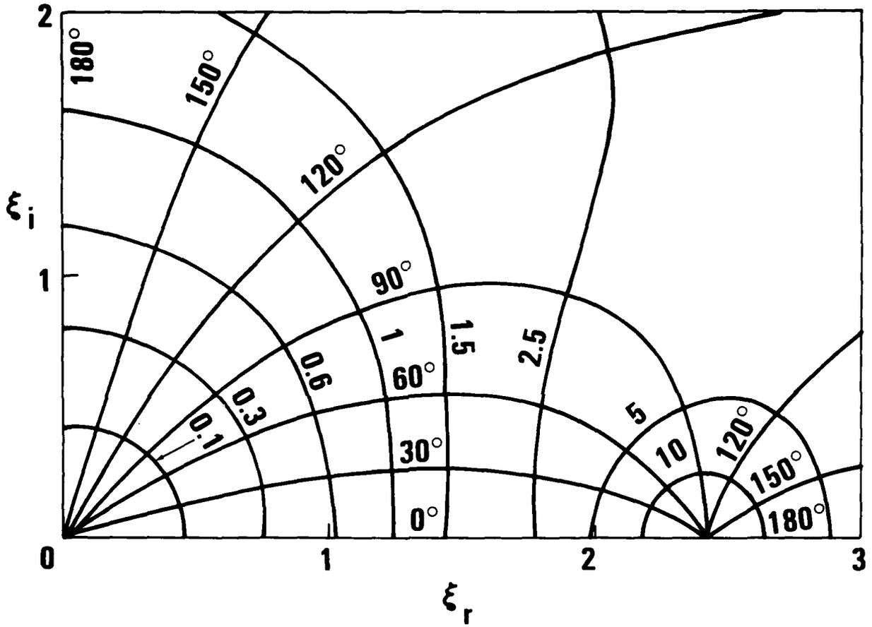
FIGURE 1 CONTOURS OF CONSTANT PHASE ANGLE  $\phi$  AND MODULUS  $f$  [EQ. (18)] IN THE COMPLEX PLANE  $\xi = (\xi_r, \xi_i)$  FOR  $n = 1$  RADIAL MODE NUMBER.
