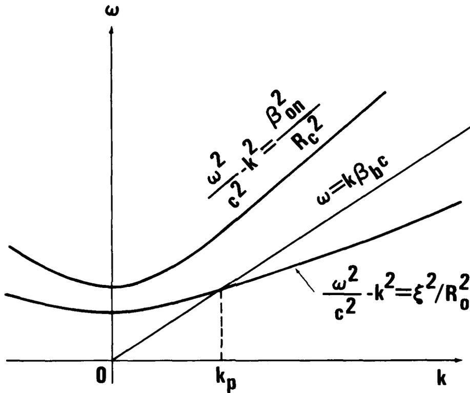
FIGURE 12 SKETCH OF  $\omega = (k^2 c^2 + \beta_{on}^2 c^2 / R_c^2)^{1/2}$  VERSUS  $k$  (CORRESPONDING TO PERFECTLY CONDUCTING WAVEGUIDE) AND  $\omega = (k^2 c^2 + \xi^2 c^2 / R_0^2)^{1/2}$  VERSUS  $k$  (CORRESPONDING TO AN ARBITRARY WALL IMPEDANCE  $Z$ ). THE STRAIGHT LINE  $\omega = k \beta_{bc}$  IS THE FREE-STREAMING MODE.
