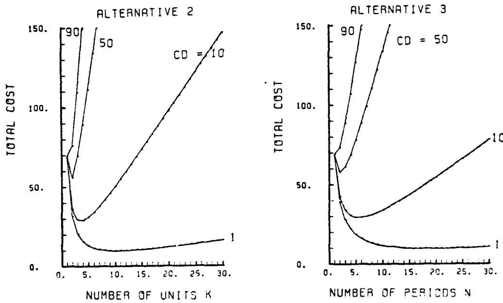
Figure 5. Total Cost Curves as a function of CD and the Decision Variables for  $p=4.5$ .
