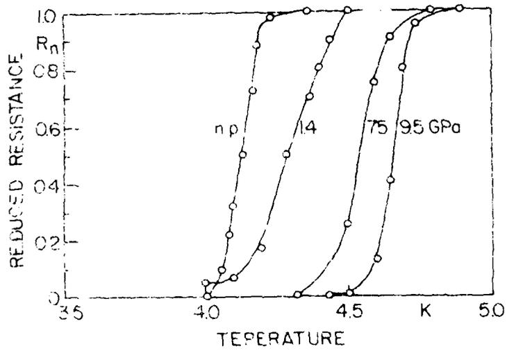
Fig.22b. Transition temperature of Ti + 11.5 at% Mo as a function of pressure.
