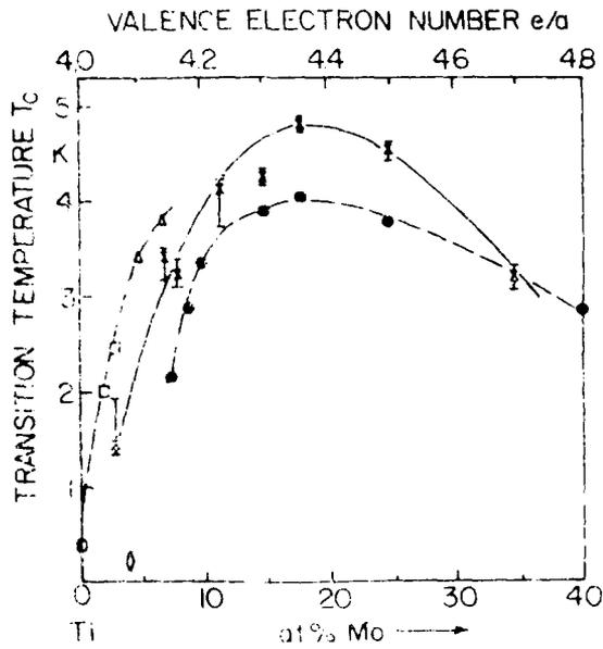
Fig.21. Transition temperature of Ti-Mo-alloys
