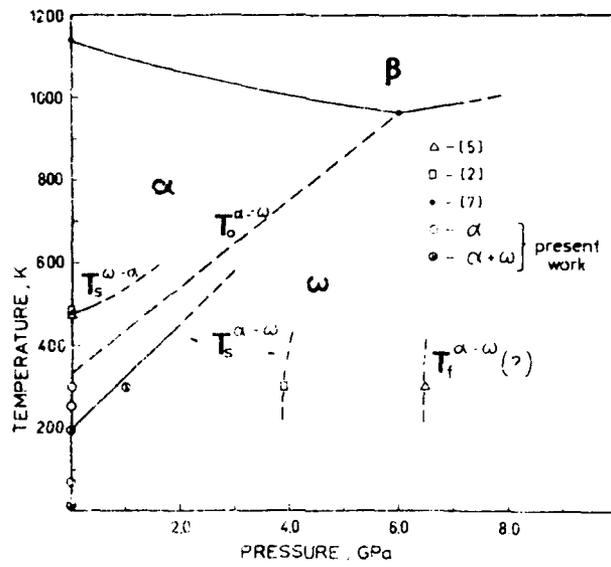
Fig.24. T-P diagram for Zirconium.
