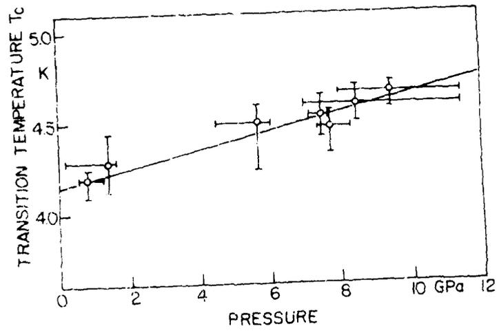
Fig.22a. Transition curves of Ti + 11.5 at% Mo under pressure.
