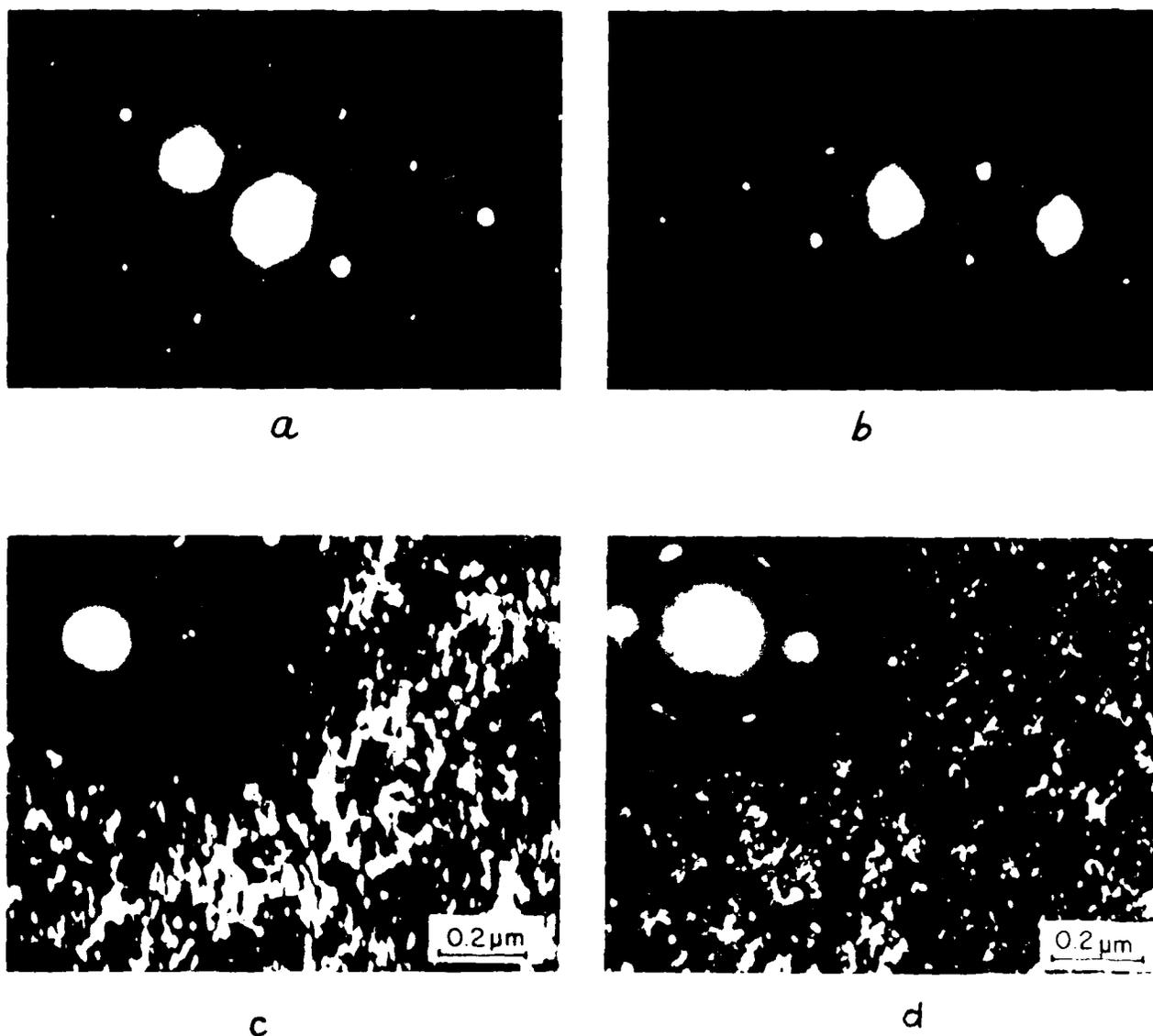
Fig.11 a) Diffuse scattering observed in the electron diffraction pattern of the as-quenched Ti-18% Mo alloy. b) Paired Kikuchi lines observed in the electron diffraction pattern of the as-quenched Ti-20% Mo alloy. TEM dark field micrographs of the c) Ti-18% Mo and d) Ti-25% Mo showing the particles of  $\beta$ -like phase in the  $\alpha$  matrix after hps 4.5GPa. E.A.  $[100]_{\alpha}$  for Ti-18% Mo and E.A.  $[111]_{\alpha}$  for Ti-25% Mo.
