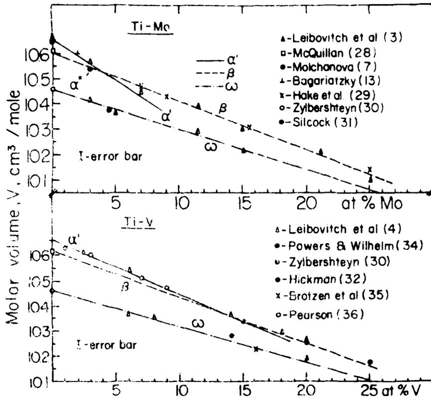
Fig.3. The molar volume of bcc( $\beta$ ) and omega ( $\omega$ ) structures in the Titanium-Molybdenum and Titanium-Vanadium Systems at one atmosphere and 300°K after various authors.
