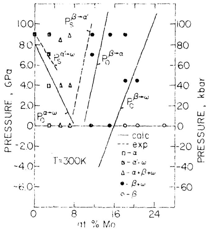
Fig 4. Summary of Experimental data on Phase Stability of Ti-Mo Alloys (3,4) as a Function of Pressure at 300K Compared with Results Computed from Equations (34)-(36).
