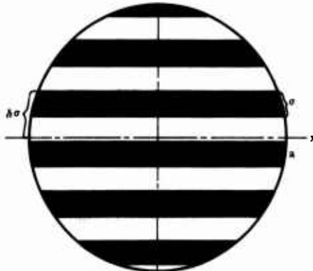
Fig. 17-16. Translating bar-reticle circular aperture and rotating scene at aperture center.
