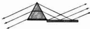
Fig. 20-19. Wadsworth constant-deviation, prism-mirror arrangement. The beam enters the prism at minimum deviation and emerges displaced but not deviated from its original direction [20-9].
