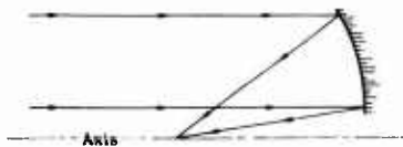
Fig. 9-19. The Herschel mount with off-axis aperture to remove the image from the incoming beam.
