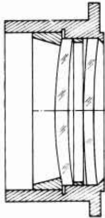
Fig. 9-48. Refractive optical system [9-12].
