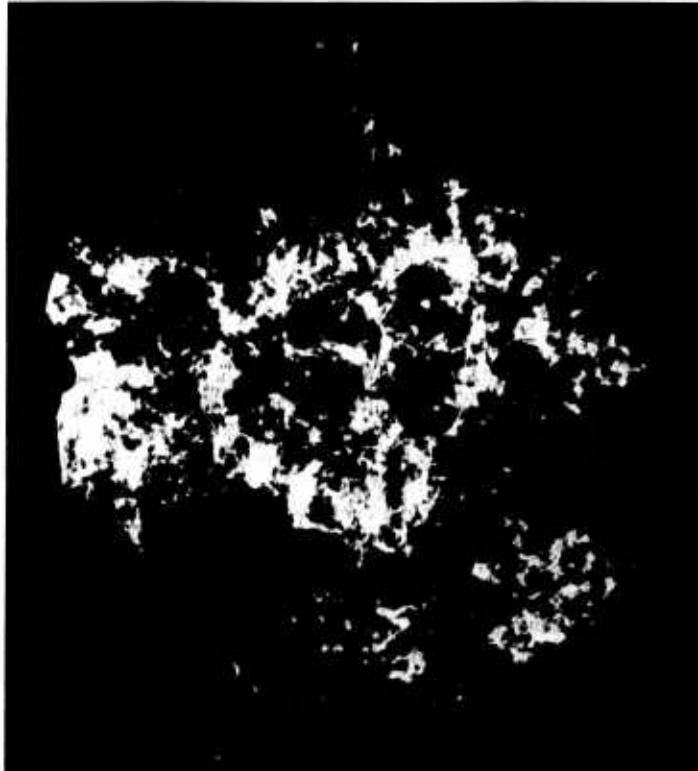
(a) Photograph of a typical laser beam profile after propagation through a long turbulent path.
