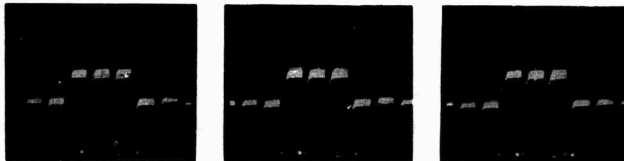
Fig. IV-1. Demonstration of low-signal charge transfer inefficiency. Nine charge packets, each about 110 electrons, are shown after 1008 transfers through device. Each photograph is time exposure of about 200 traces, with noise level near 10-rms electrons.
