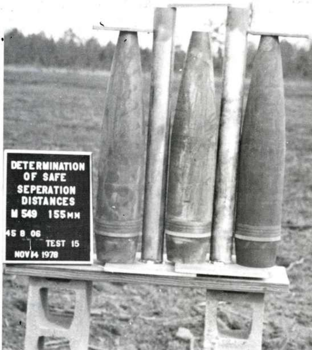
Figure 4. Test array, shielded single projectile
