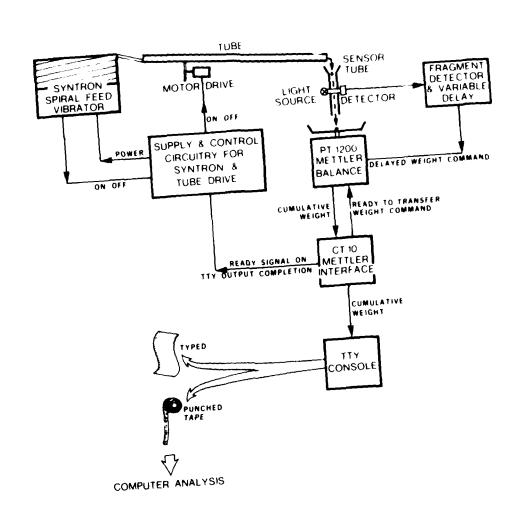
FIG. 5 - Schematic diagram of automatic fragment weighing machine.
