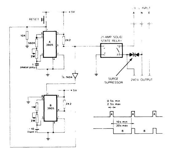
FIG. 1 - Circuit diagram of variable duty cycle timer for the vibrating spiral sorter.
