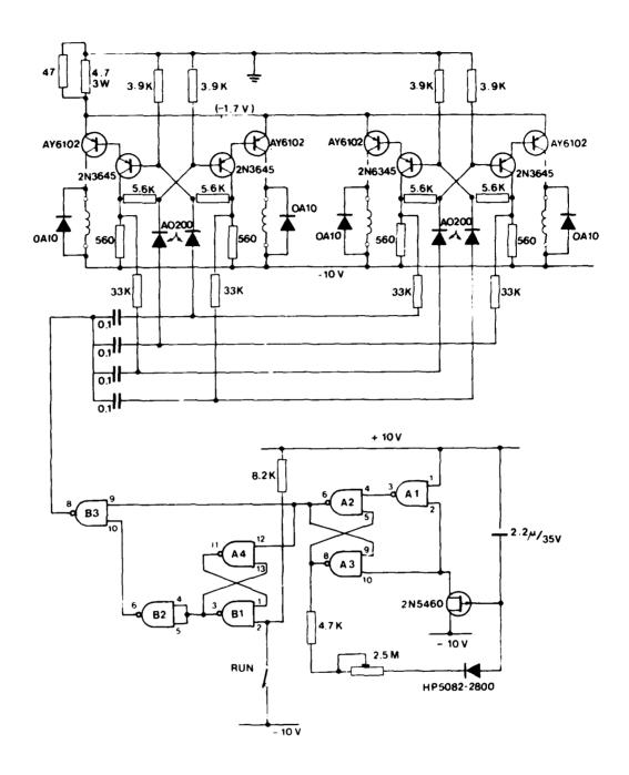
FIG. 2 - Variable speed feed tube motor drive.
