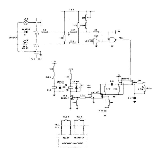
FIG. 4 - Fragment sensor and data transfer circuitry.
