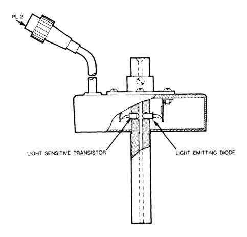
FIG. 3 - Light beam fragment sensor.
