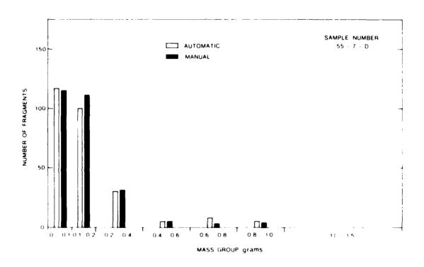
FIG. 9 - Comparison of manual and automatic fragment counts in individual mass groups for cylinder 55-7-D.
