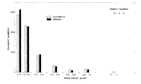
FIG. 8 - Comparison of manual and automatic fragment counts in individual mass groups for cylinder 55-6-D.
