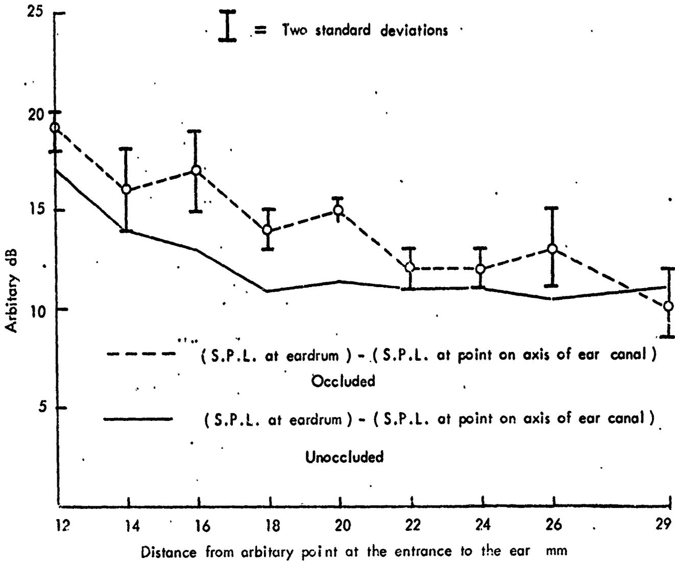
Fig 6 Showing difference in the resonance pattern in KEMAR's ear canal between the occluded and unoccluded states
