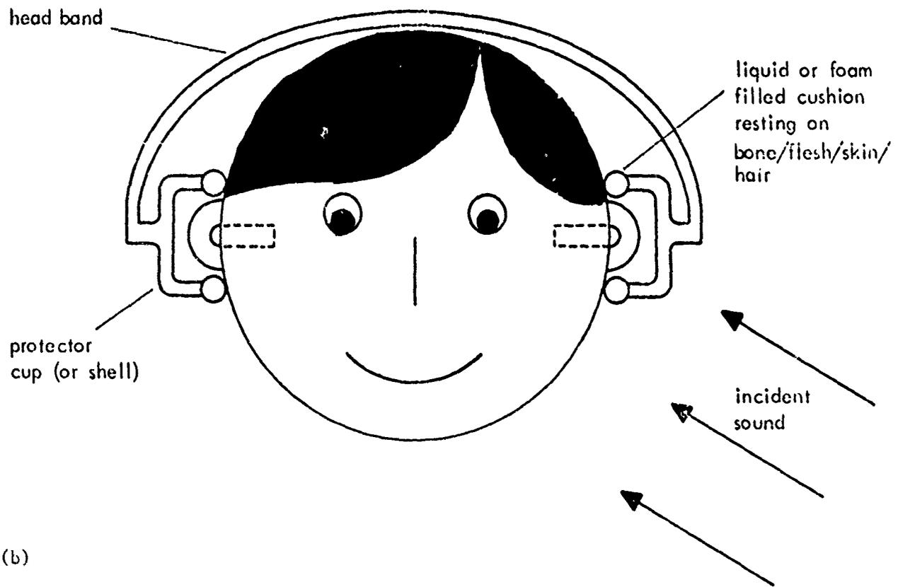
Fig 1 Illustrating important factors in the measurement of the attenuation of circumaural hearing protectors
