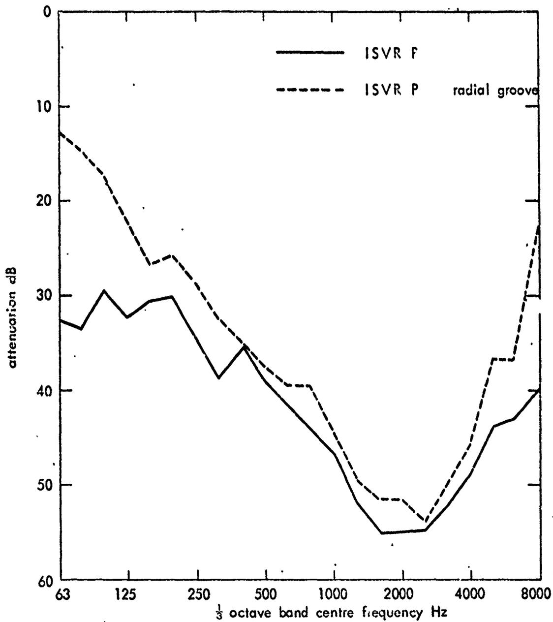
Fig 7 Effect on attenuation of radial groove (liquid-filled cushion)
