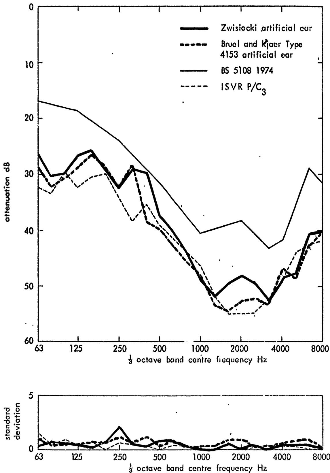
Fig 5 Attenuation spectra as measured by four methods
