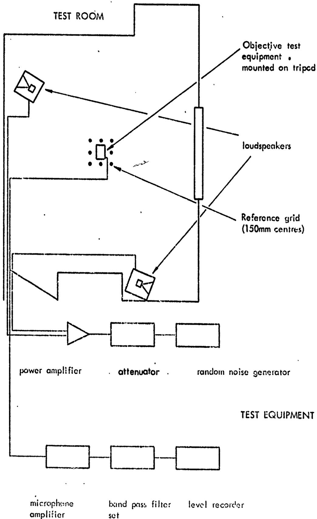
Fig 2 Showing experimental layout used for objective tests
