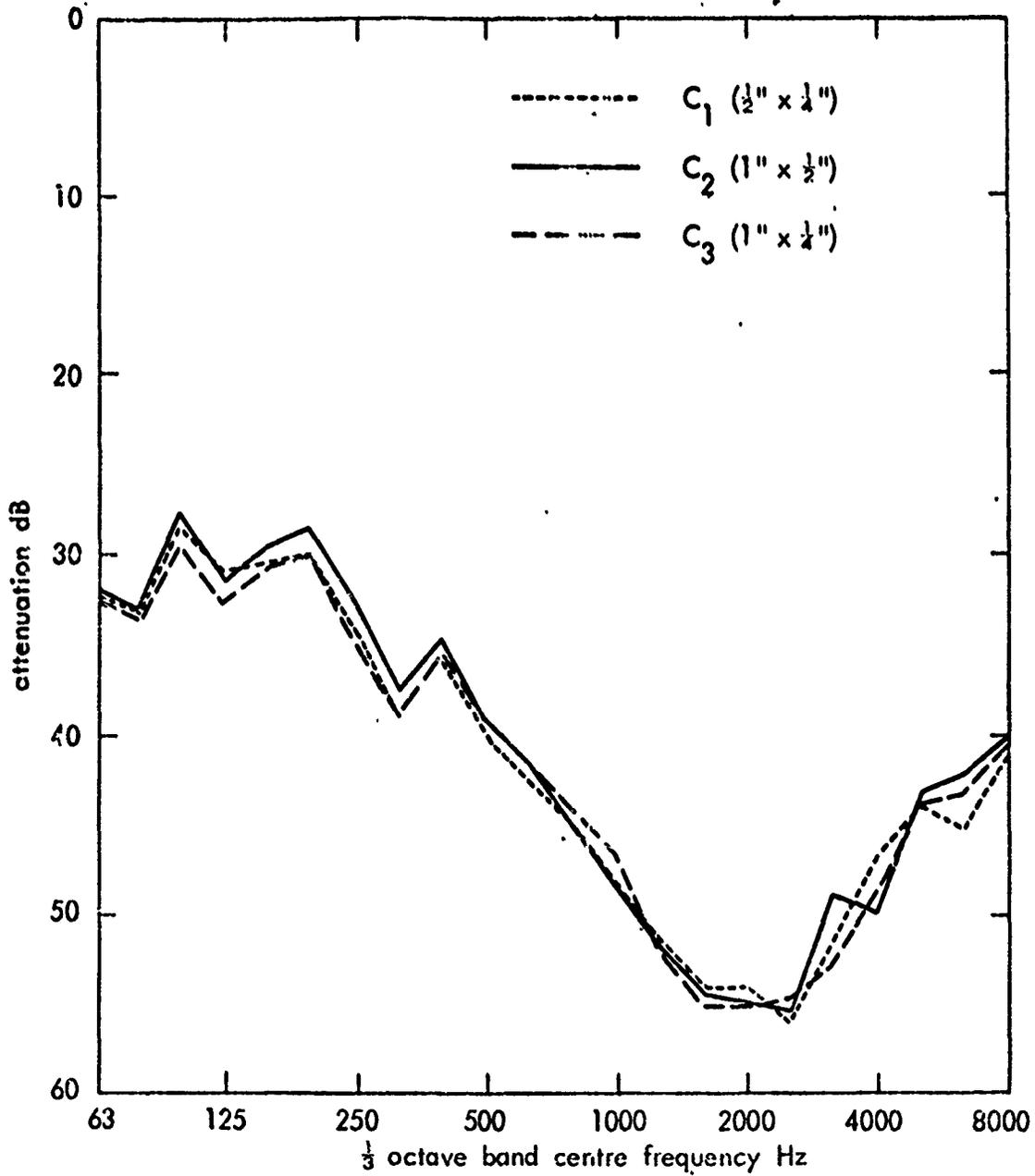
Fig 4 Attenuation spectra-measured using three couplers of different geometries
