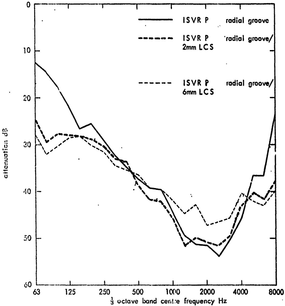
Fig 8 Effect of skin simulant on attenuation (liquid-filled cushion).
