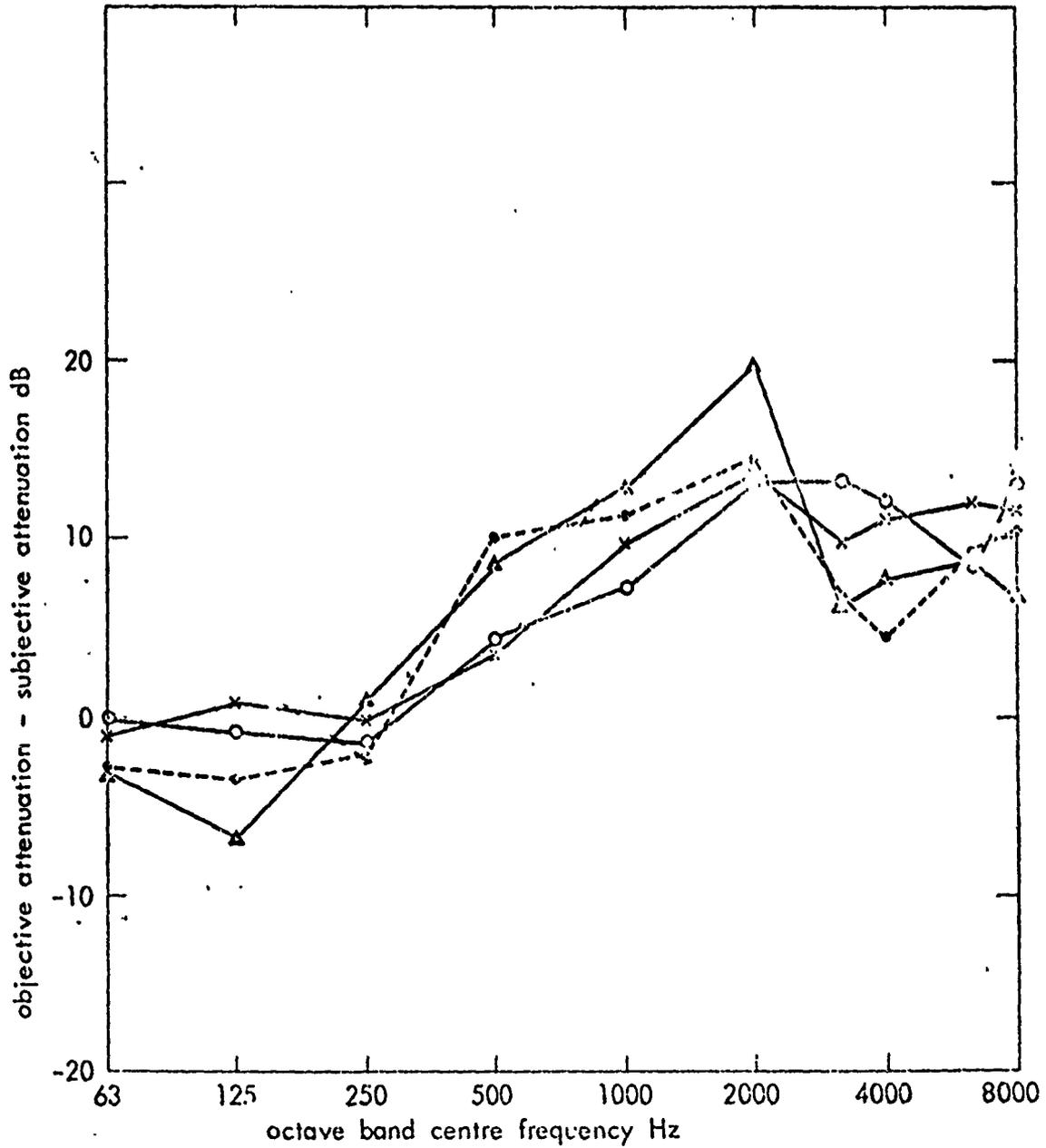
Fig 11 Spectrum of difference between objective and subjective attenuation measurements for earmuffs with foam-filled cushions
