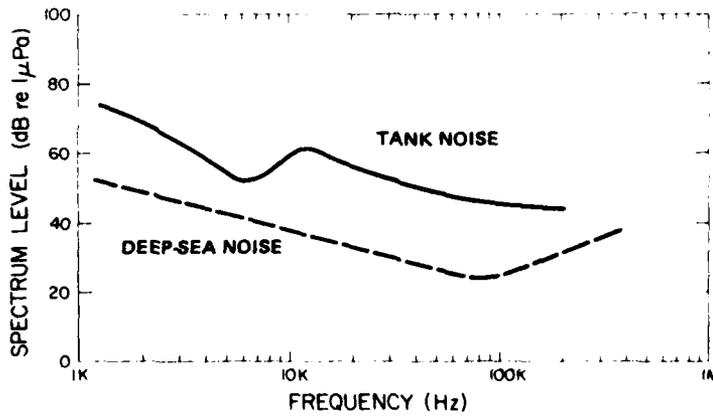
Fig. 15 — Spectrum of ambient noise in the tank
