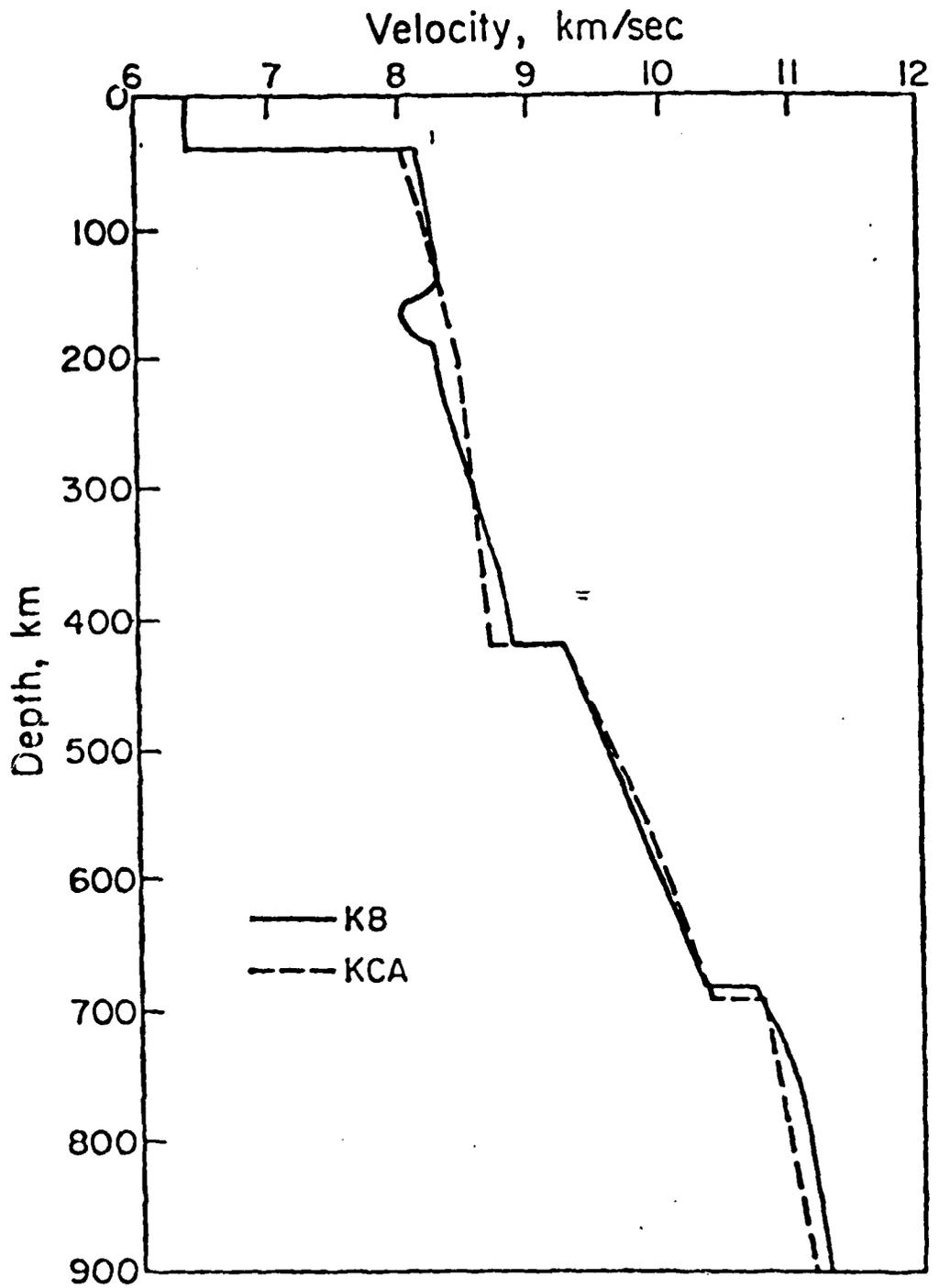
Figure 5. Model K8 (derived by Given and Helmberger, 1980) and Model KCA (King and Calcagnile, 1976) for northwest Eurasia. (Modified from Given and Helmberger, 1980.)
