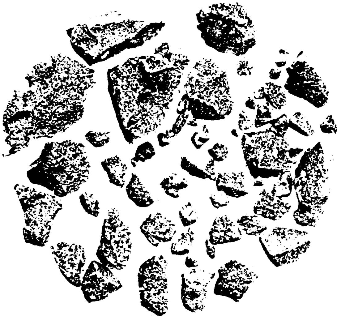
*Figure 1. Composition B fragments found in closed bomb following sudden pressure relief.*
