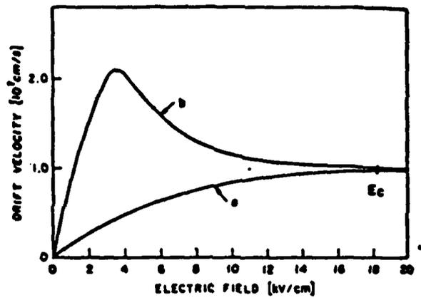
Fig. 1 Velocity-field characteristics in GaAs and silicon.<sup>1)</sup>
