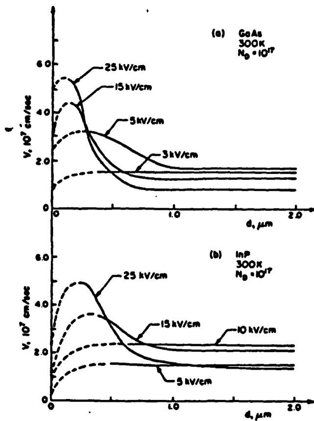
Fig. 2 Instantaneous velocity vs distance for 300°K,  $N_a = 10^{17}$ ; (a) GaAs, (b) InP.<sup>2</sup>
