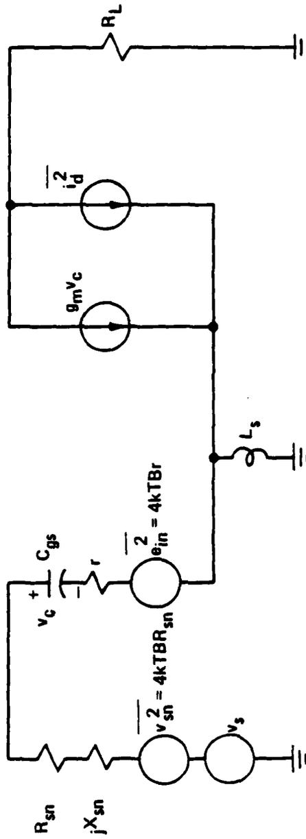
Fig. 13 Simple FET noise model which includes the effect of source inductance.
