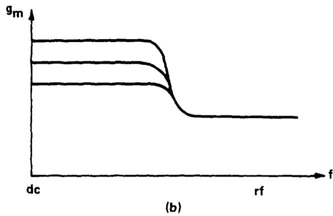
Fig. 16 Variation of  $g_m$  with frequency illustrating dispersion.
