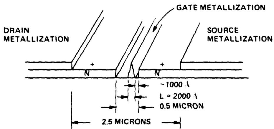
Fig. 7 Cross section of gate channel area.
