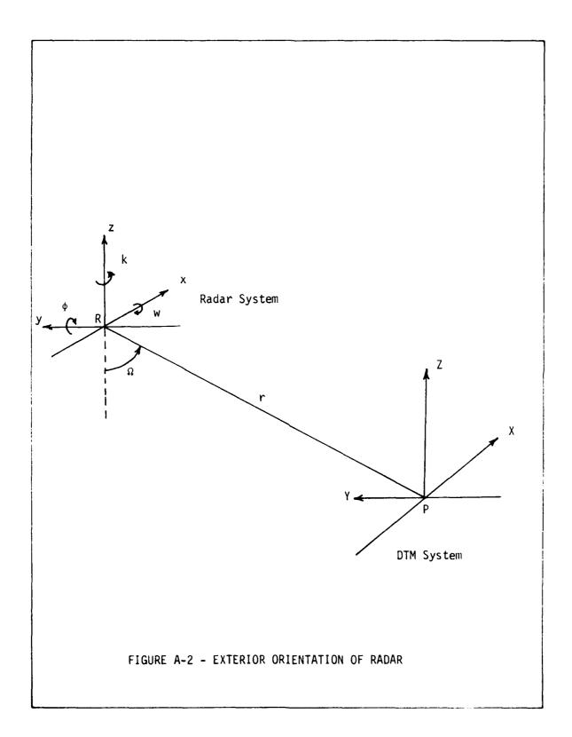
In order to provide a complete sample computation such as that carried out in the study it will be necessary to refer to a sketch of the ficticious locations of radar and ground position. (See Figure A-2).
