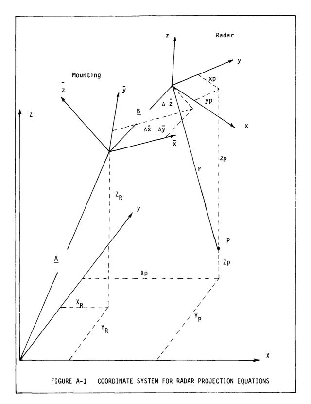
A simplification of equation (A-3) will now be made by assuming that the sensor is parallel and coincident with the mount. In this case B becomes a unit matrix and  $\Delta \bar{X}$  is zero.
