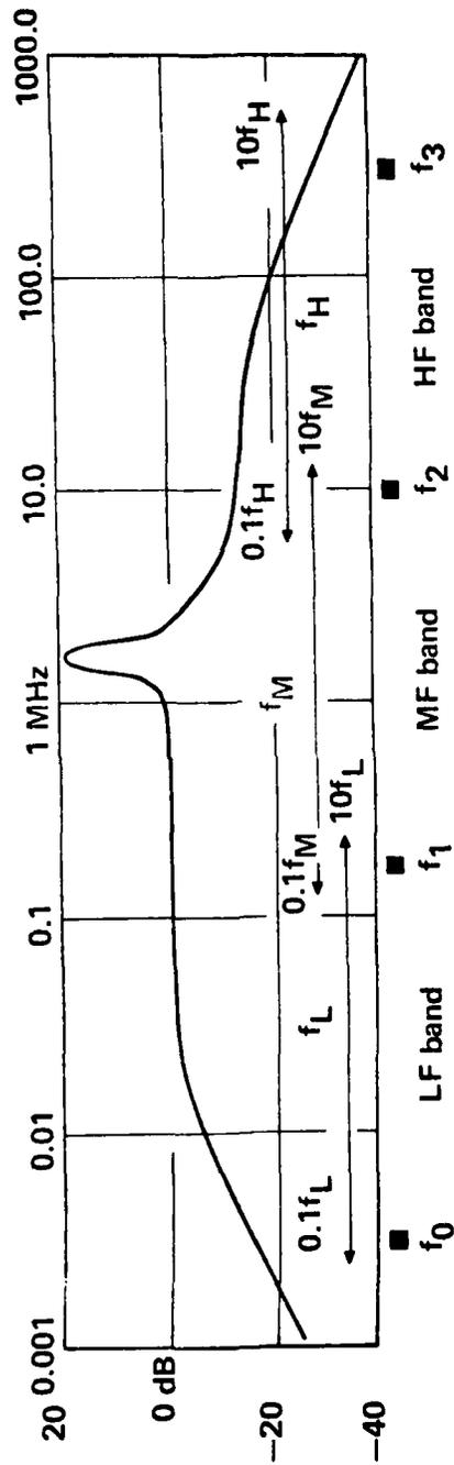
Fig. 10 Definition of LF, MF and HF frequency bands
