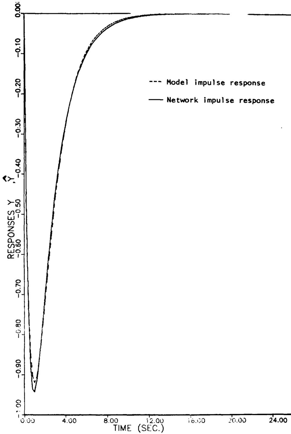
Fig. 8a Comparison of network and model impulse responses.
