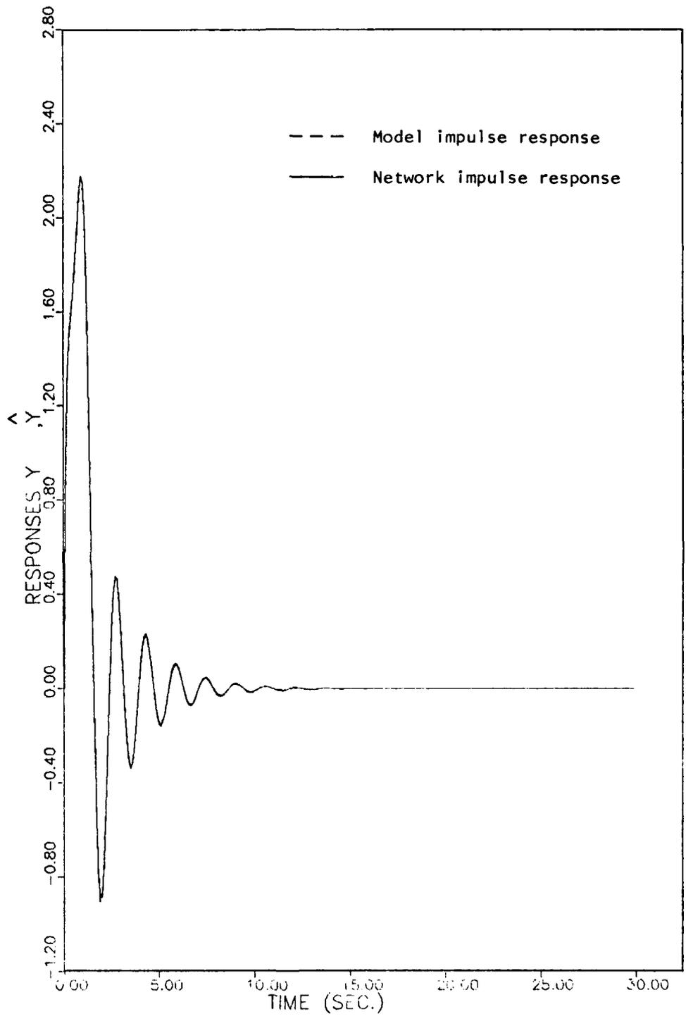
Fig. 6. Comparison of network and model impulse responses
