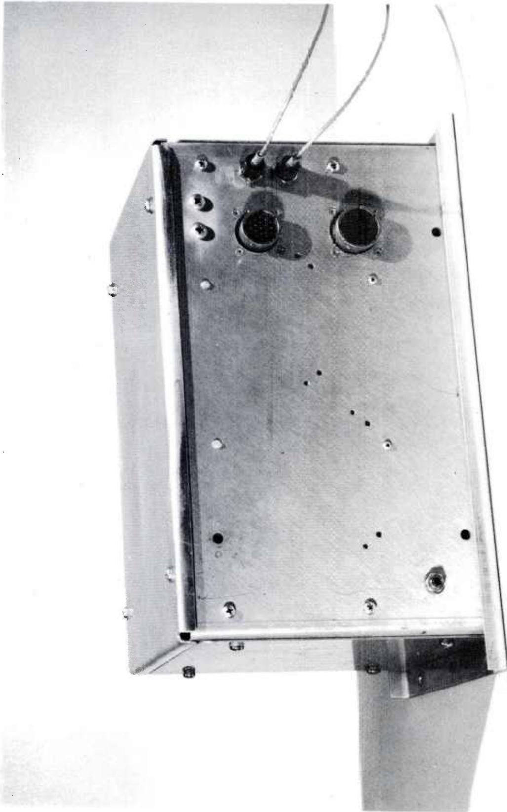
Figure 2-9. Microcomputer Unit With Fiber Optic Cables Attached
