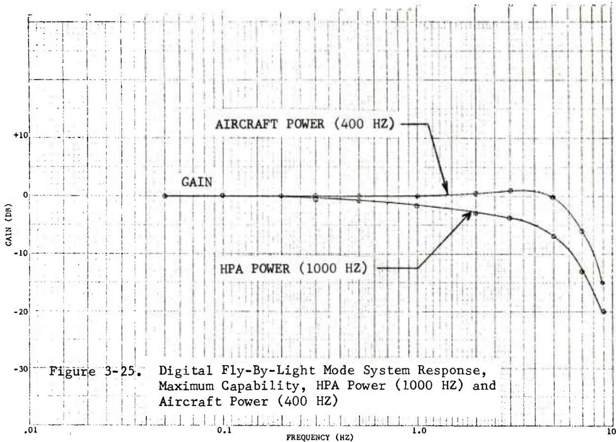
Figure 3-25. Digital Fly-By-Light Mode System Response, Maximum Capability, HPA Power (1000 HZ) and Aircraft Power (400 HZ)
