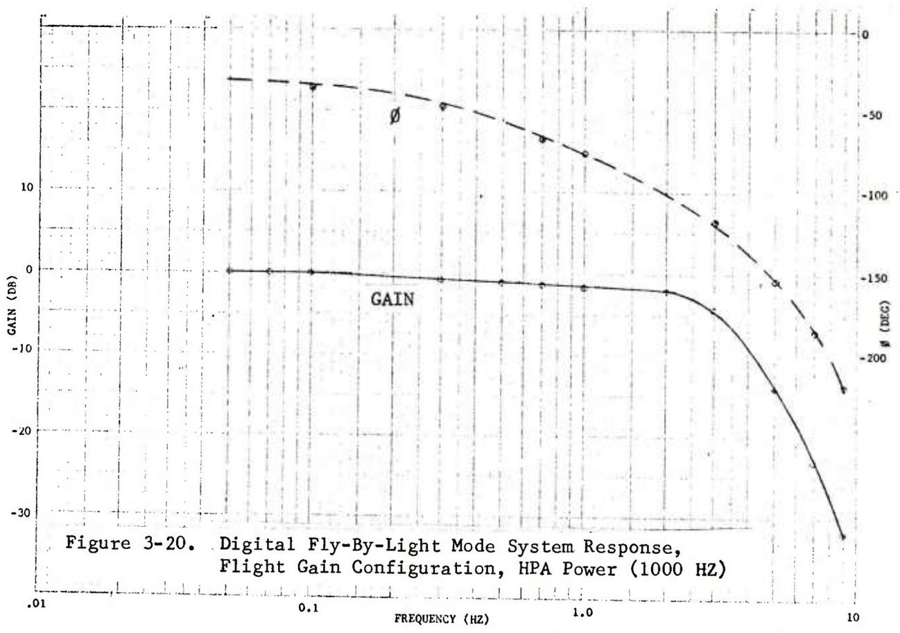
Figure 3-20. Digital Fly-By-Light Mode System Response, Flight Gain Configuration, HPA Power (1000 HZ)
