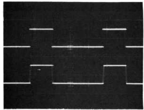
Figure 3-27. Temperature Test Fiber Optic Loop Input and Output Waveforms
