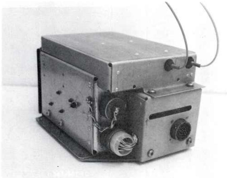
Figure 2-6. EDU With Fiber Optic Cables Attached
