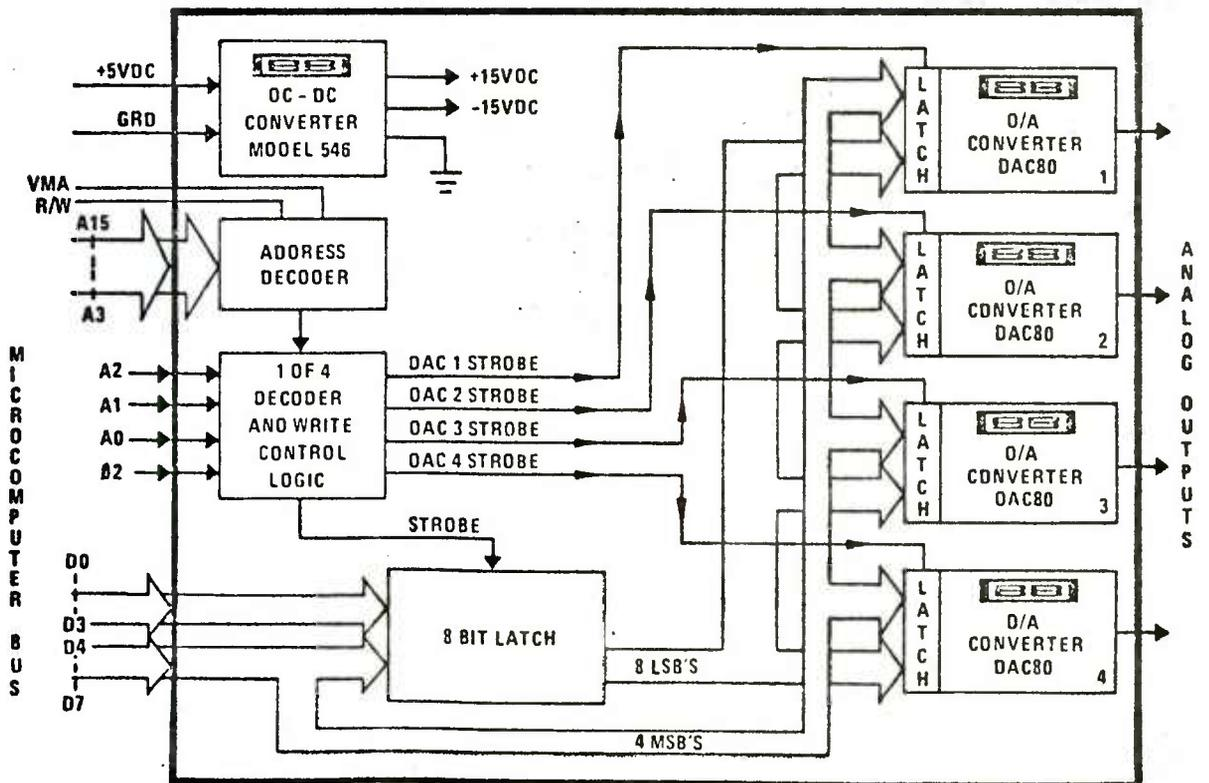
Figure A-5. Digital to Analog Converter - MP7104
