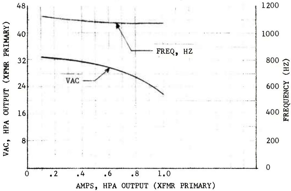
Figure 3-6. HPA VAC & Frequency Versus HPA Output Current
