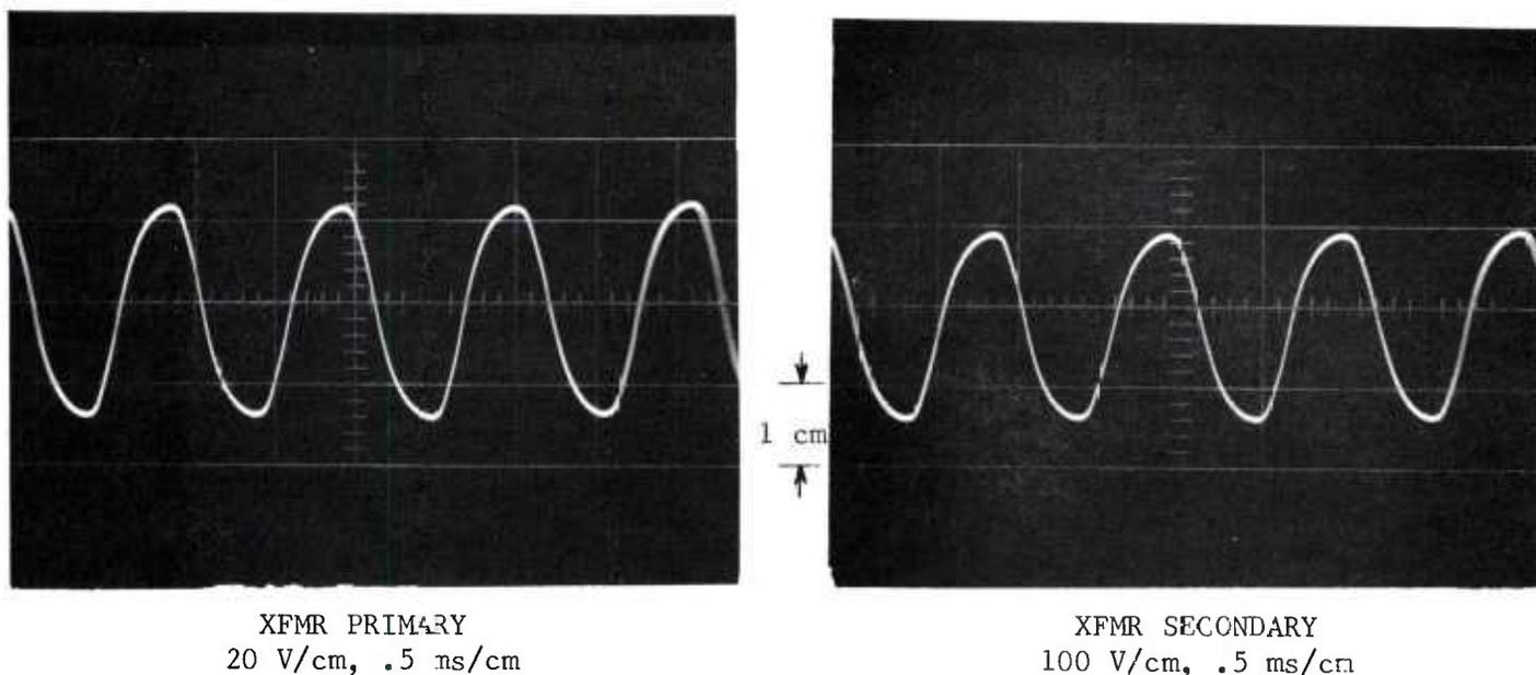
Figure 3-12. Transformer Primary and Secondary Voltage Waveforms, 2500 PSI FPA  $\Delta P$
