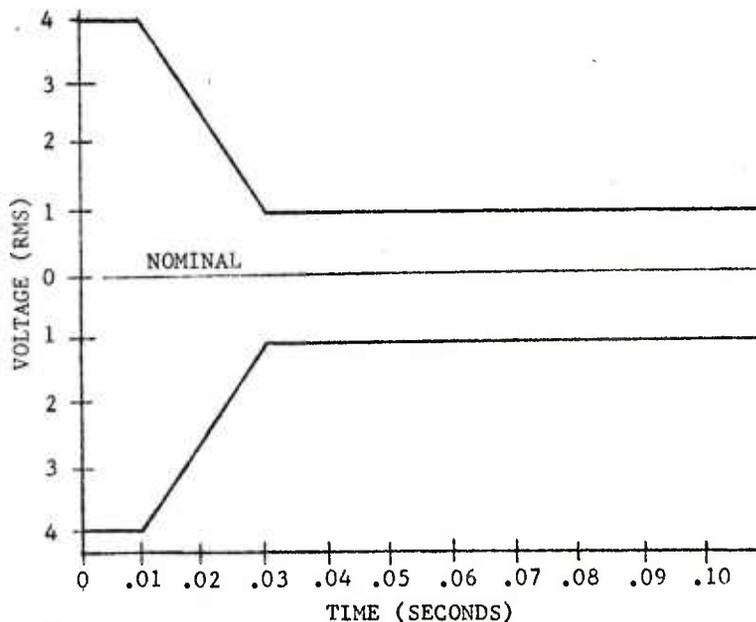
Transient and Steady State Regulation @ Rated Capacity
