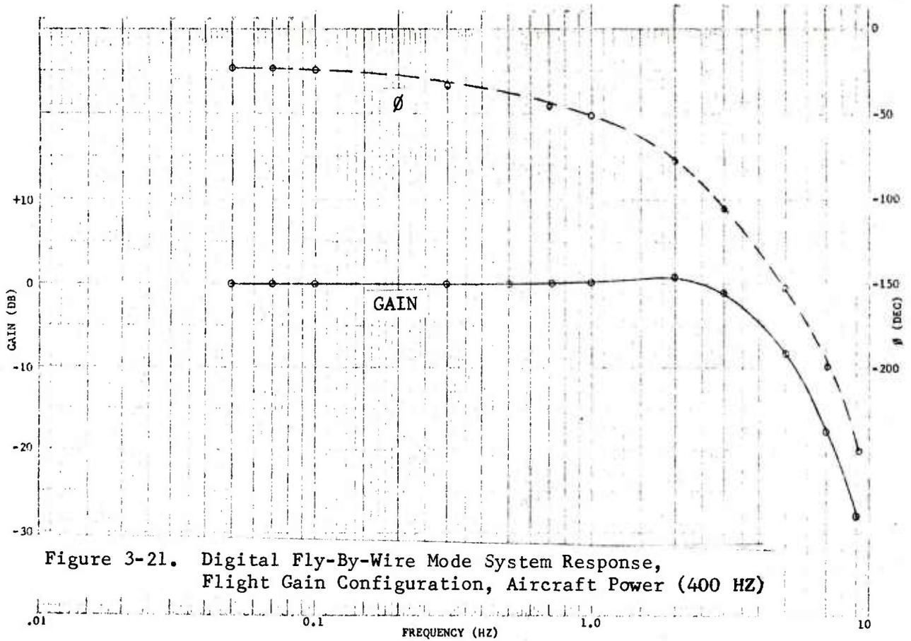
Figure 3-21. Digital Fly-By-Wire Mode System Response, Flight Gain Configuration, Aircraft Power (400 HZ)
