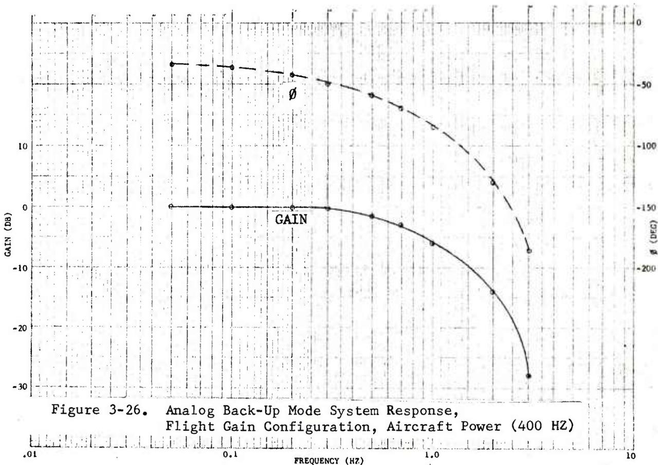
Figure 3-26. Analog Back-Up Mode System Response, Flight Gain Configuration, Aircraft Power (400 HZ)
