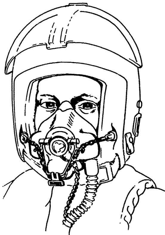
Figure 2.1; GENERAL VIEW OF TYPICAL HELMET/MASK COMBINATION
