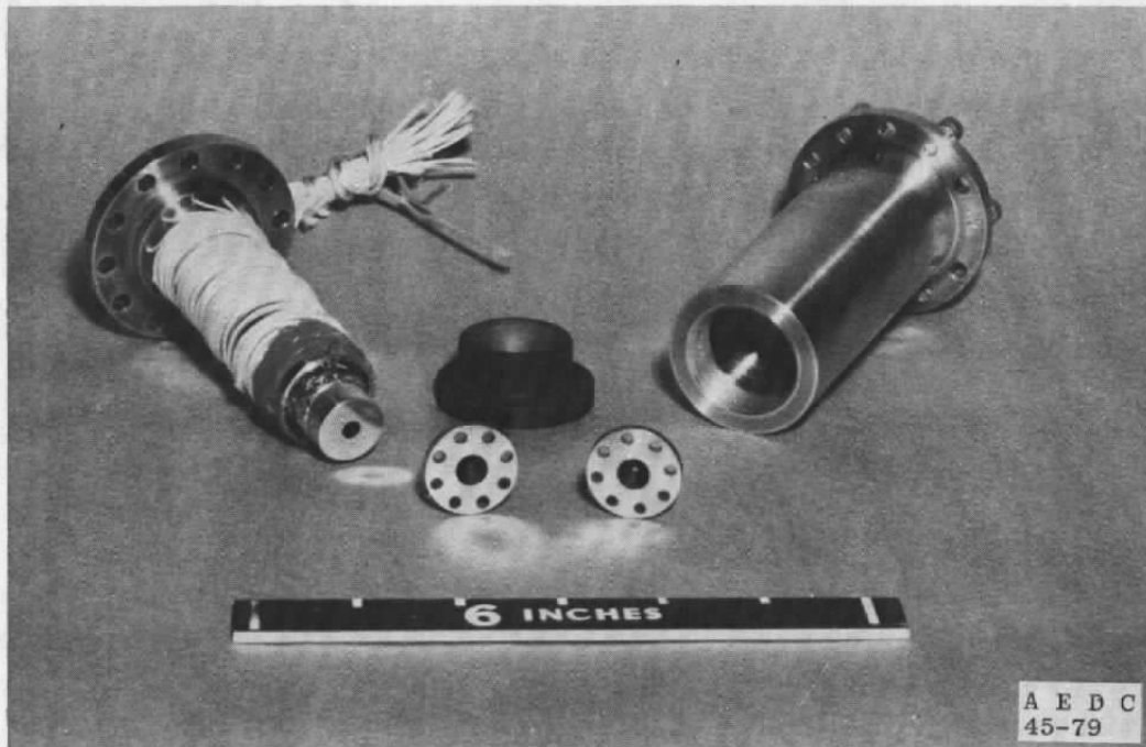
Figure 11. AEDC-VKF standard infrared source components.
