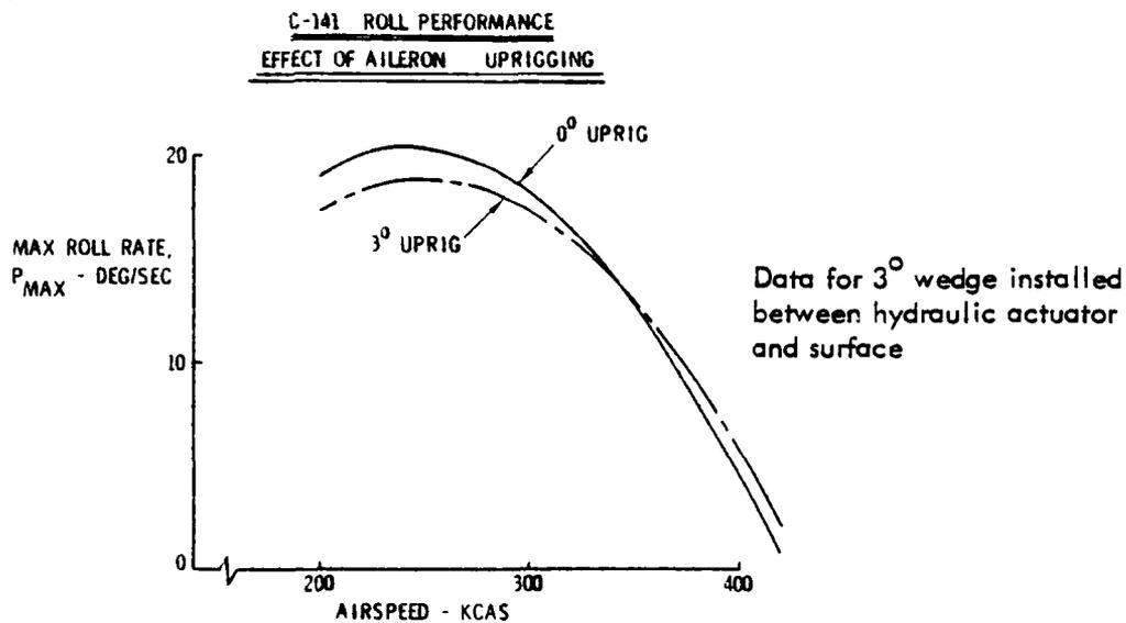
The data indicates less than a  $1.5^\circ$  per second change in maximum roll rate. Roll power should not be affected as total aileron deflection (both left and right) is not changed. Similar results are expected for the  $6^\circ$  uprig.
