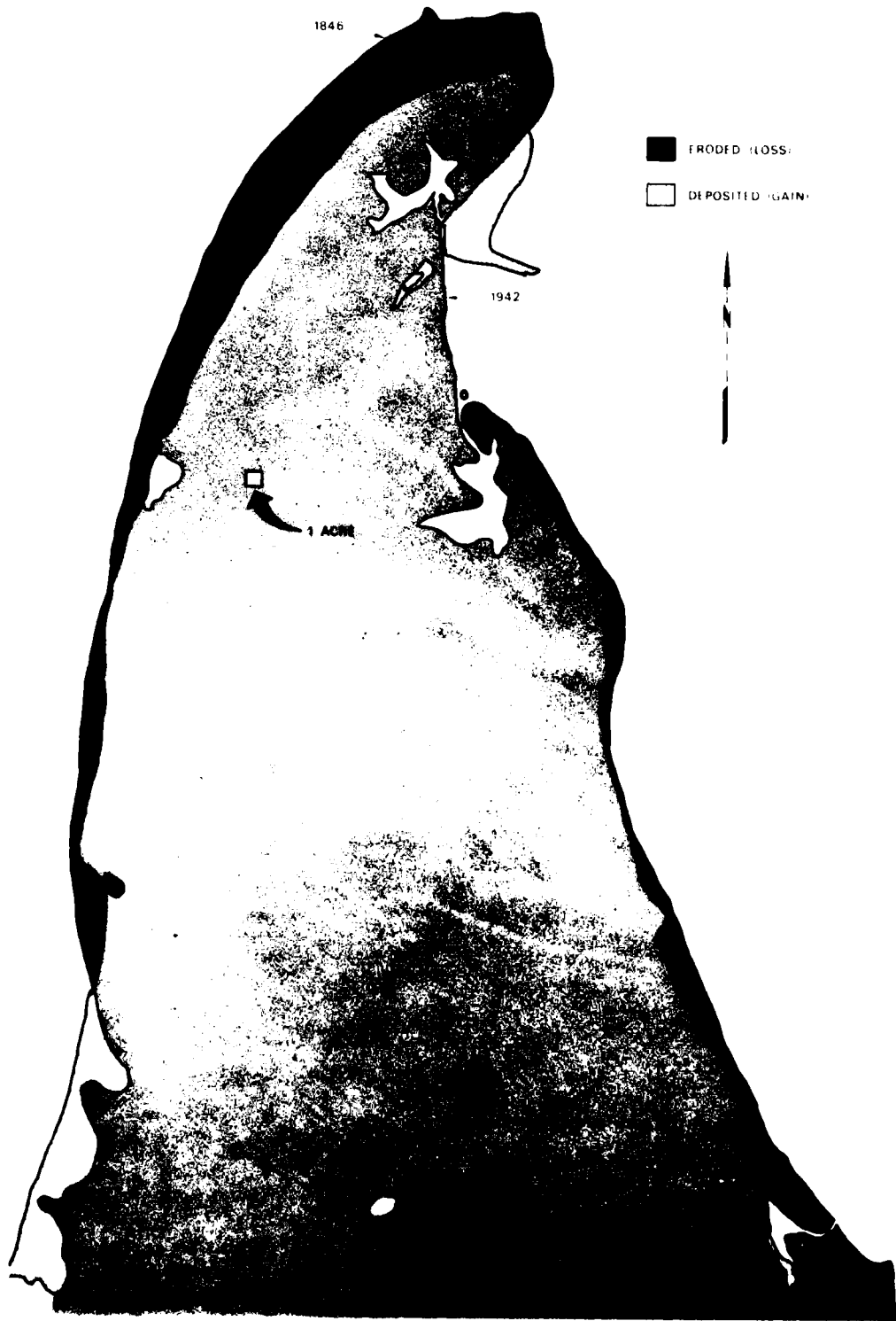
Figure 23 Shoreline erosion (black area) around Love Point at the north end of Kent Island during the period 1846 to 1942 based on measurements from old charts and aerial photographs compiled by the Maryland State Geological Survey.
