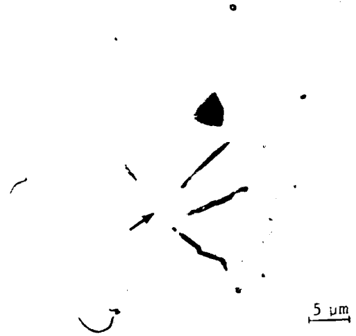
(b) Subsurface crack pattern after 1 \mu\text{m} of material removal. Indentation gone, radial cracks visible (arrow indicates locus of indent apex), no median cracks visible.
