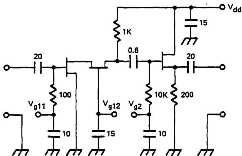
Fig. 2.2 IF amplifier schematic circuit.
