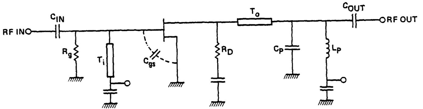
Fig. 2.11 Amplifier circuit for sensitivity analysis.
