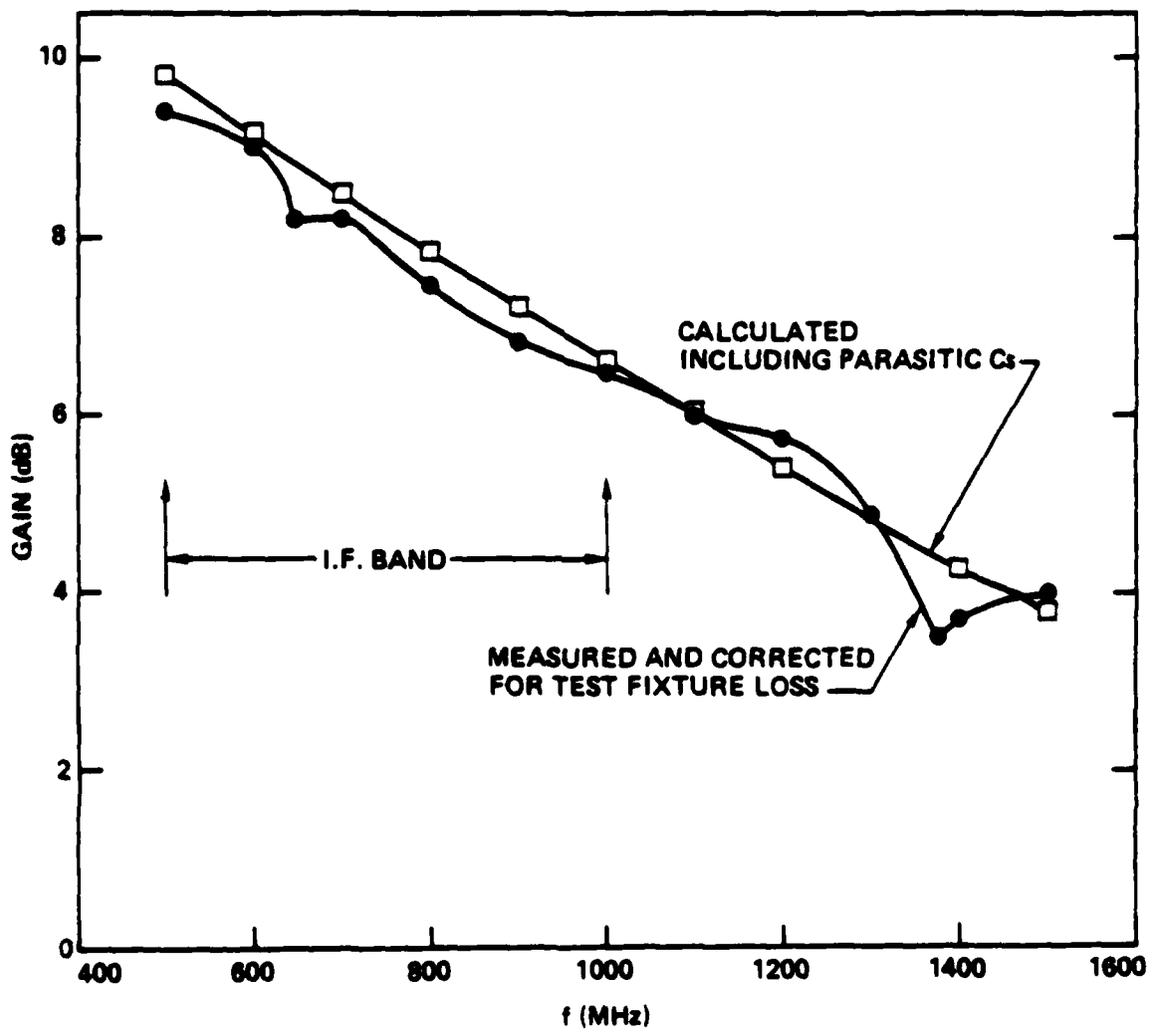
Fig. 2.6 Measured gain of IF amplifier.
