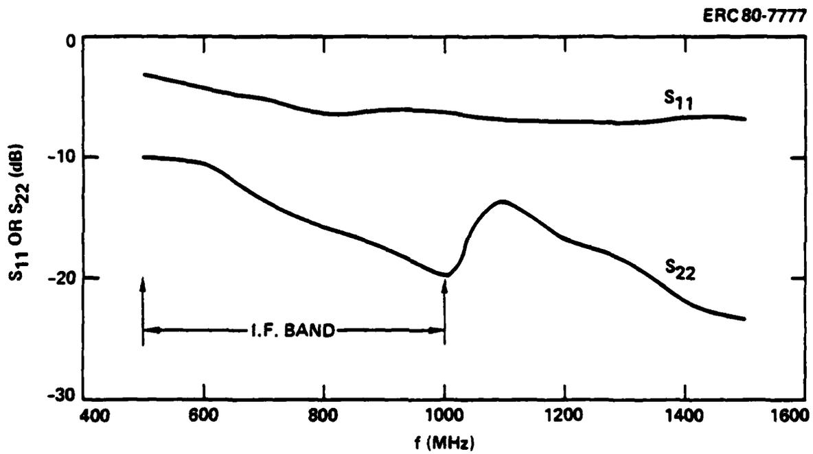
Fig. 2.7 Measured  $S_{11}$  and  $S_{22}$  of IF amplifier.
