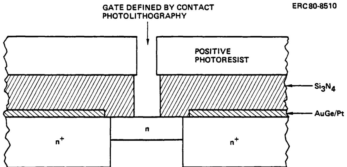
Fig. 3.3 A schematic diagram showing the nitride aided lifting process.  $\text{Si}_3\text{N}_4$  is deposited on GaAs and the gate pattern is defined in positive photoresist on top. Exposed  $\text{Si}_3\text{N}_4$  is etched in a plasma. Gate metal is then evaporated and lifted as usual.
