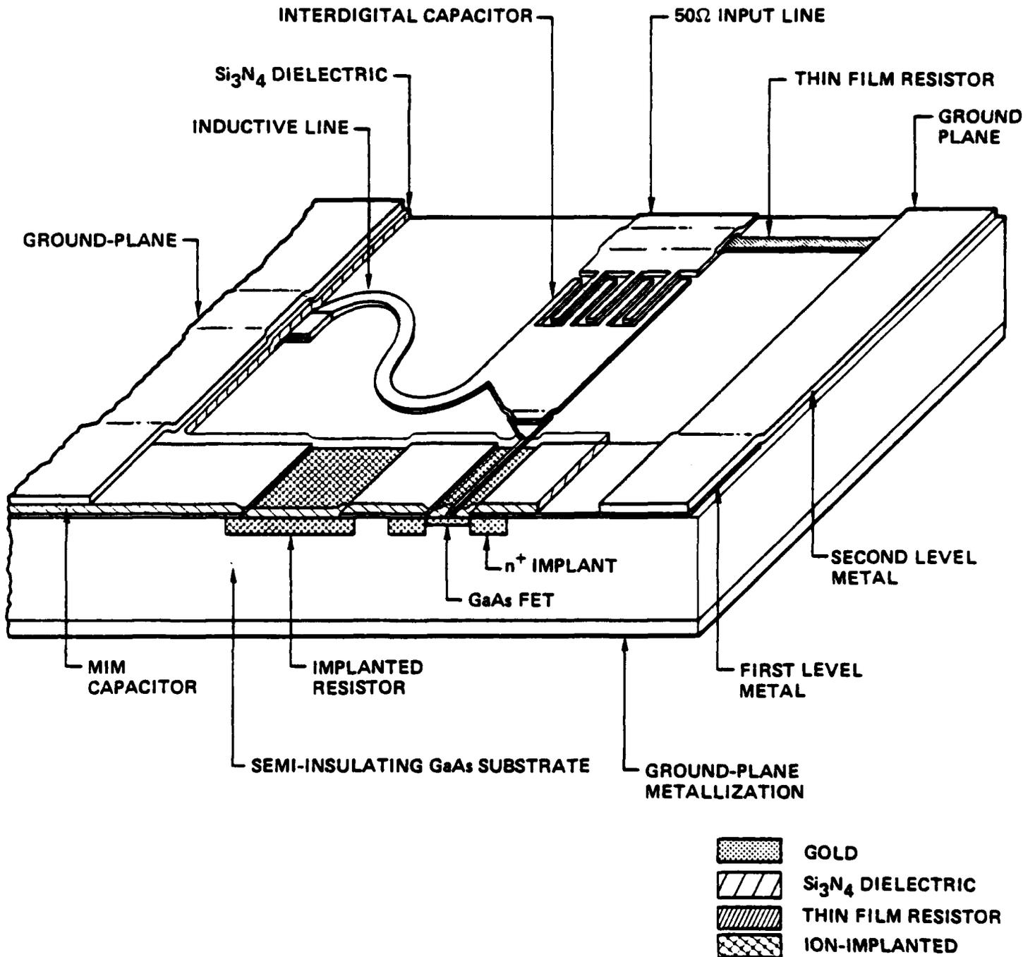
Fig. 3.1 Schematic diagram of a monolithic microwave integrated circuit.
