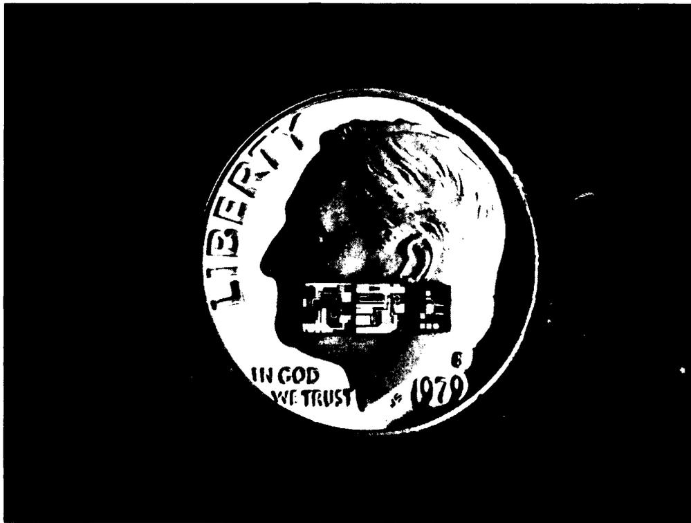
Fig. 2.1 This photograph shows the RF preamplifier (left), the FET mixer (center), and the IF amplifier (right) on the face of a dime. The preamp and the mixer are each  $2.5 \times 2.5 \text{ mm}^2$  and the IF amplifier is approximately  $2 \times 2 \text{ mm}^2$  in size.
