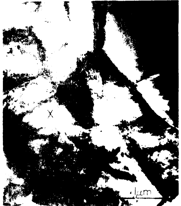
Figure 7. Transmission electron micrograph of Ti-30% W alloy heat treated at 810°C (1500°F) and water quenched showing \alpha -Ti (labeled X) in Ti.
