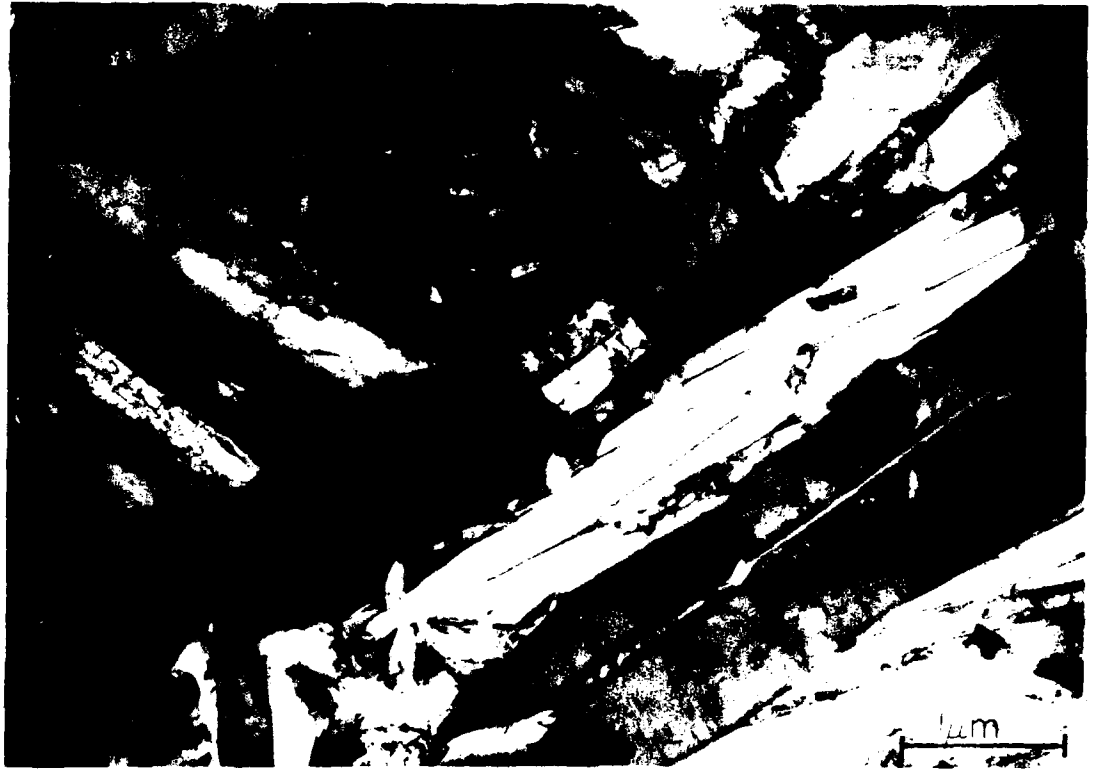
Figure 22. Transmission electron micrograph of the same specimen as in Figure 21. The electron diffraction pattern indexes to be \alpha' (hexagonal) martensite.
