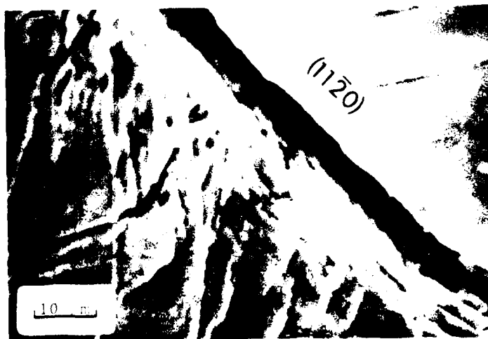
Figure 4. Severe deformation surrounding a tensile mode crack propagating on a (11\bar{2}0) plane after cycling at \pm 0.008 cyclic shear strain amplitude.
