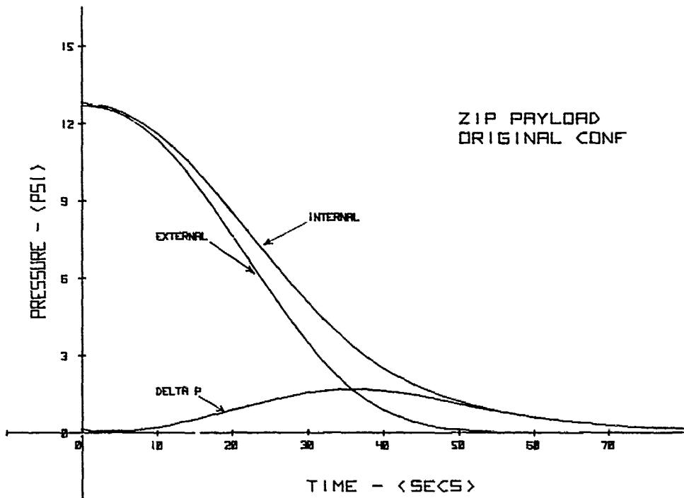
Figure 7. Program Results for ZIP Payload—Original Venting Configuration
