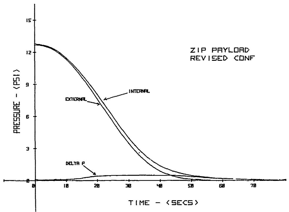
Figure 8. Program Results for ZIP Payload—Revised Venting Configuration
