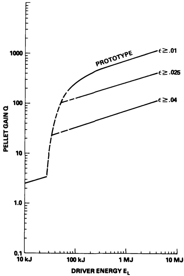
Fig. 6 - Variation of the implosion asymmetry  $\epsilon = R_i/R_o$
