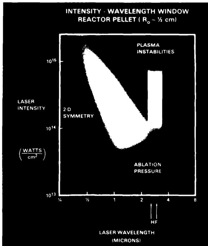
Fig. 12 — The coupling and isentrope critical elements place another barrier against the usage of high laser intensities and long laser wavelengths. The broad bandwidth of the HF laser may raise this barrier.
