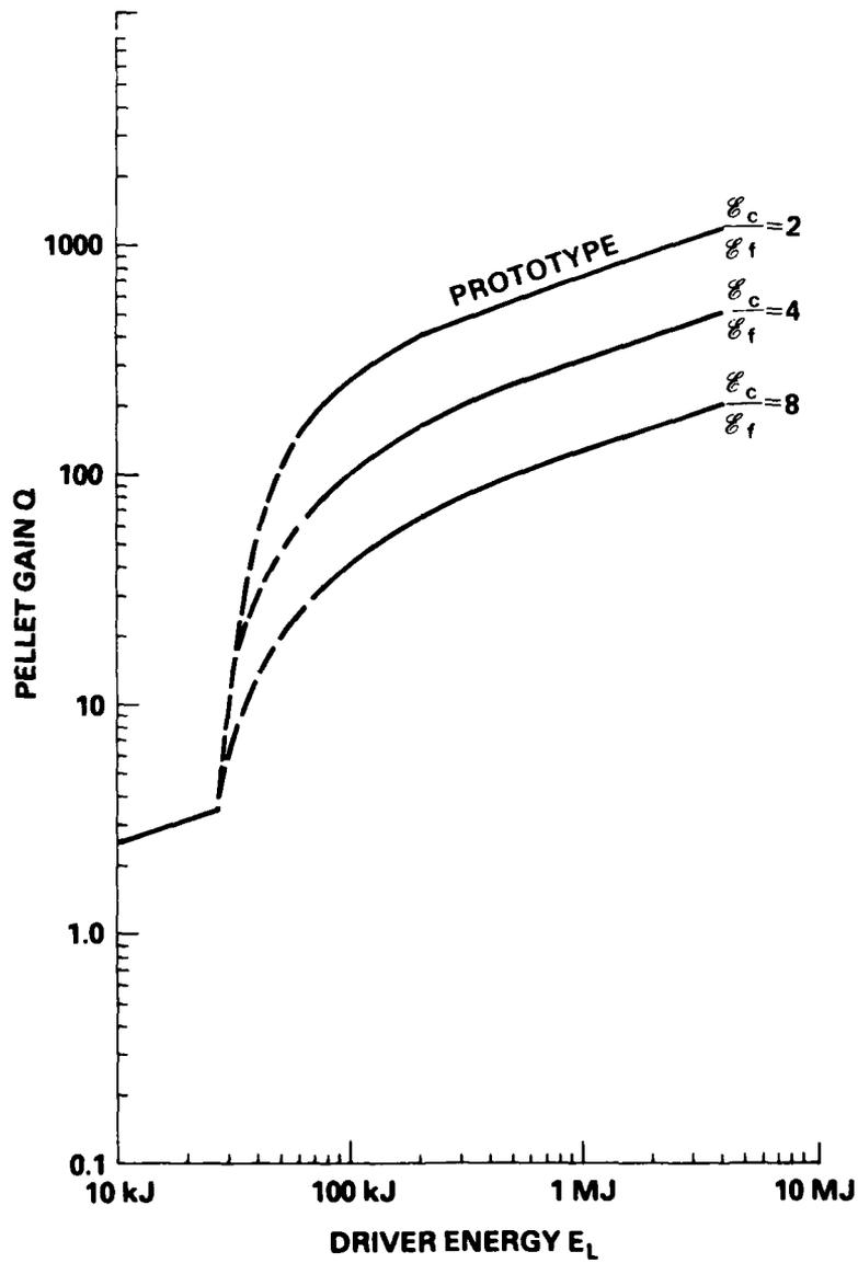
Fig. 5 — Variation of  $E_c/E_f$ , the cold fuel energy of compression, as impared to the fermi-degenerate value
