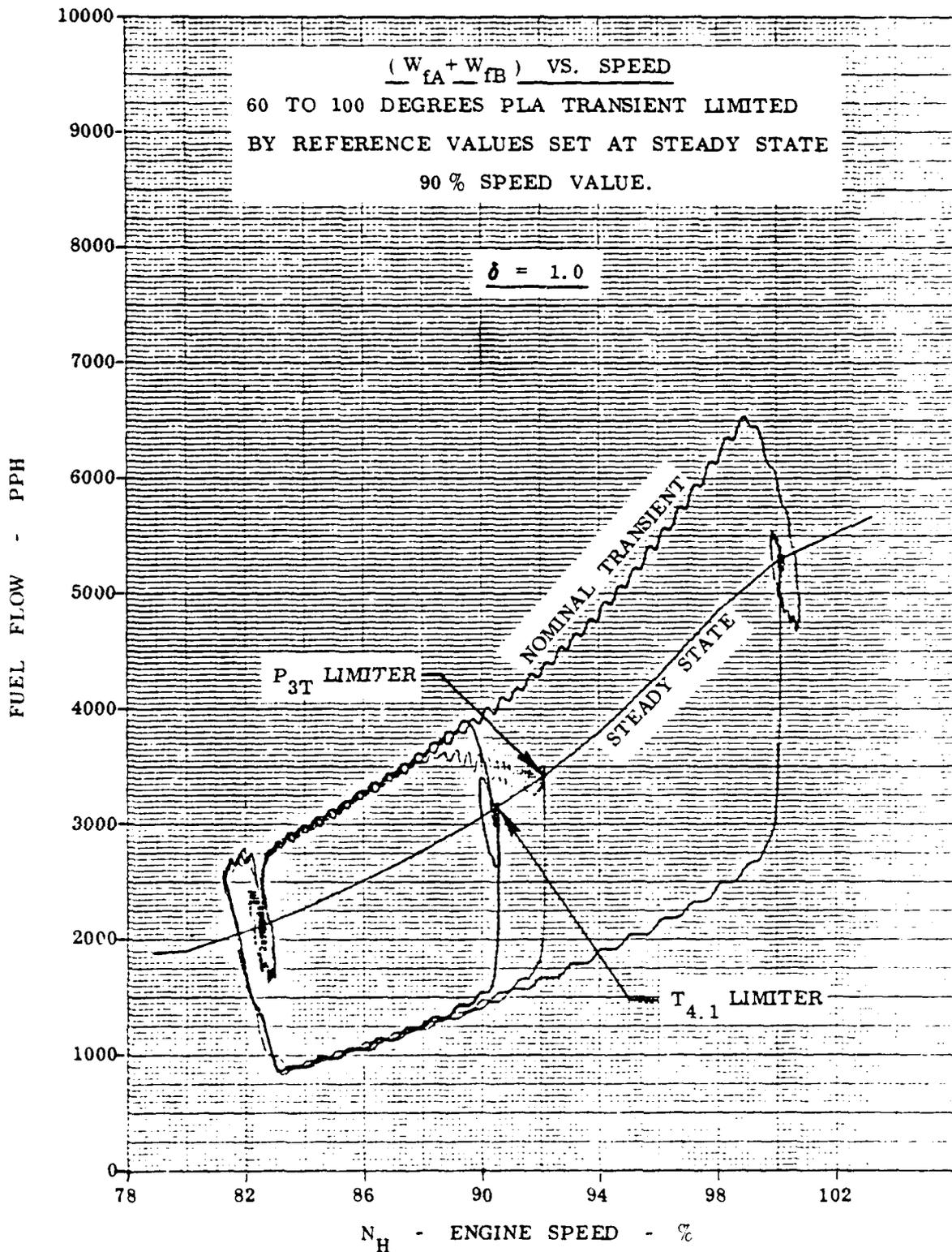
Figure 21. Parameter Limited Transients - Fixed RPR
