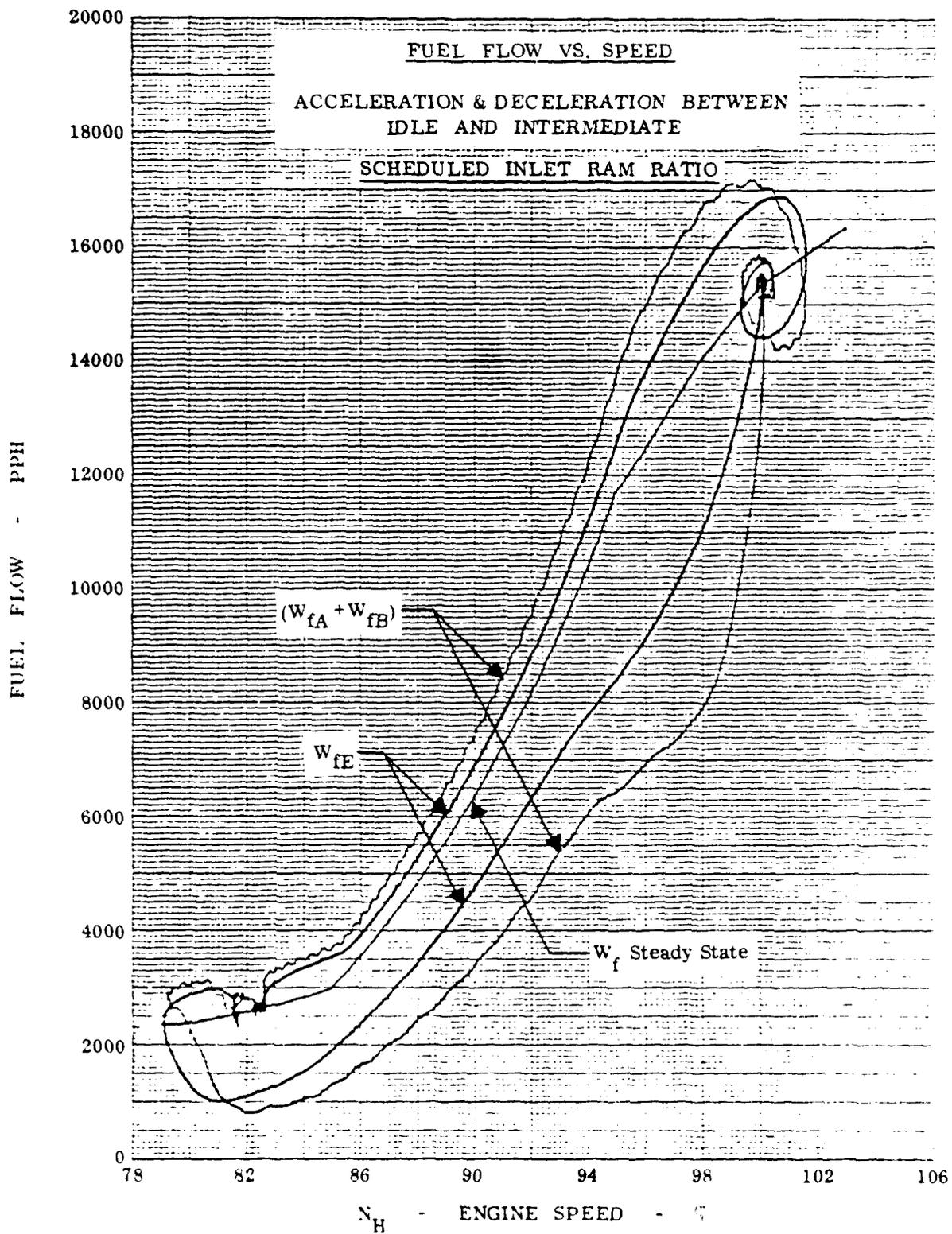
Figure 18. Transients between Idle and Intermediate - Scheduled RPR
