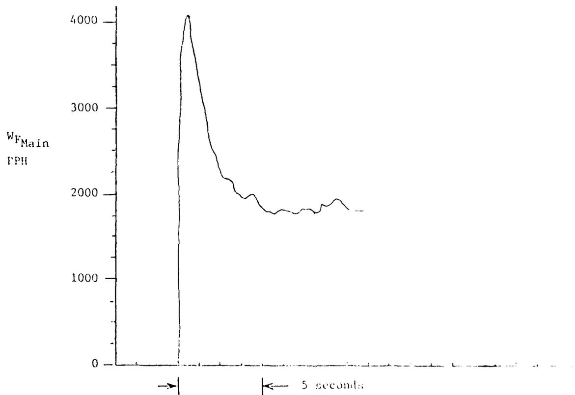
Figure 24. Stepped Responses of Pilot and Main Valves
