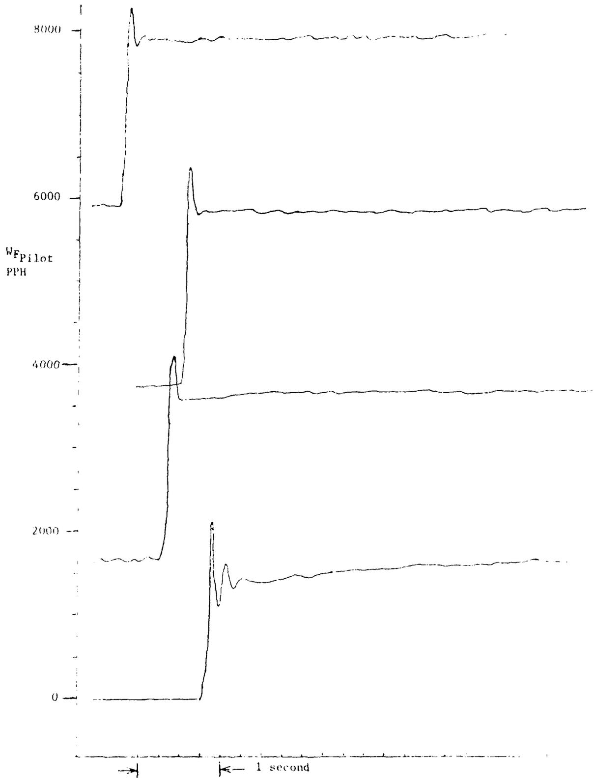
Figure 25. Pilot Valve Response - Final Configuration
