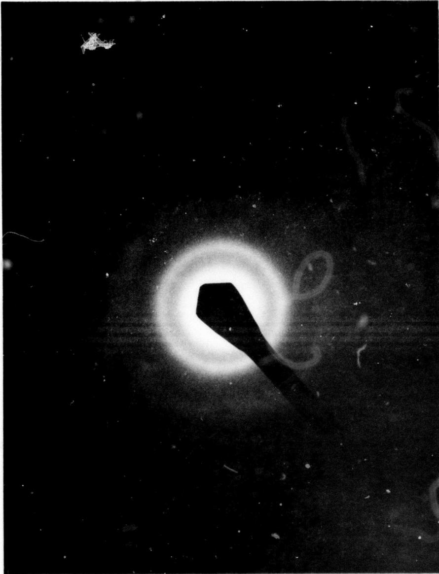
Figure 48. Selected Area Electron Diffraction Pattern, Area Denoted as A in Figures 46 and 47 of a Powder Particle and the "Matrix" Film Deposit of Fe-Ni-B-P Metallic Glass Alloy Produced by the EHD Technique
