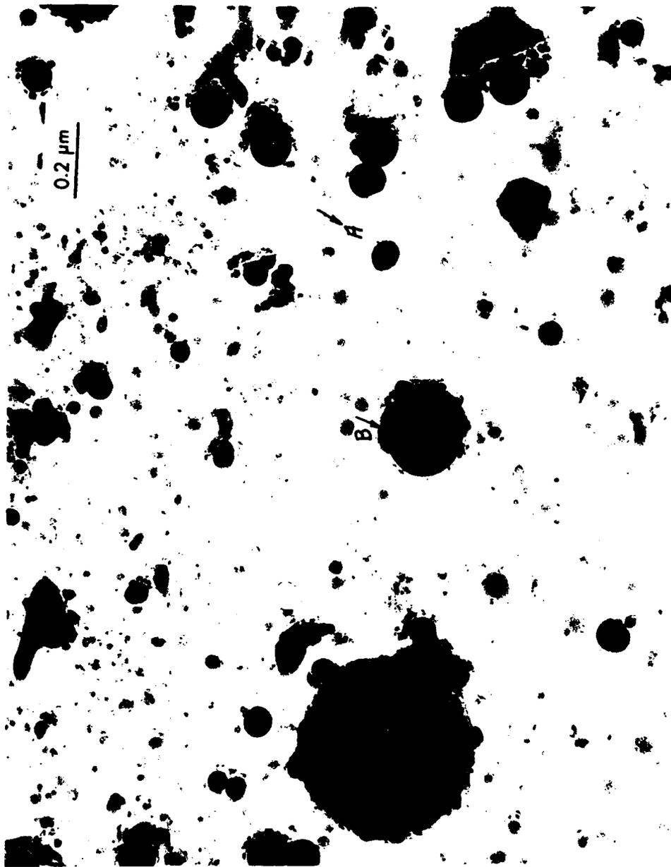
Figure 46. Transmission Electron Microscope Image of a Deposit, Fine Powders, and "Matrix" Film, of Fe-Ni-B-P Metallic Glass Alloy Produced by the EHP Technique and Collected on a Vinyl Cellulose Substrate at 74,000X.
