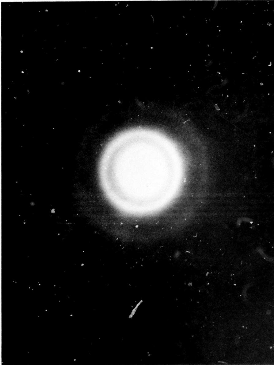
Figure 45. Selected Area Electron Diffraction Pattern, 0.3  $\mu\text{m}$  in Diameter, of the Continuous "Matrix" Film Deposit of Fe-Ni-B-P Metallic Glass Alloy Produced by the EHD Technique on a Vinyl Cellulose Substrate
