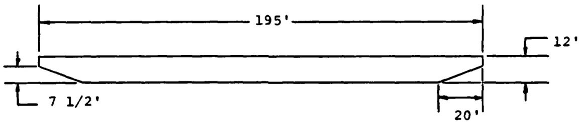
Figure 1: Full Scale Dimensions of Barge Type Tested
