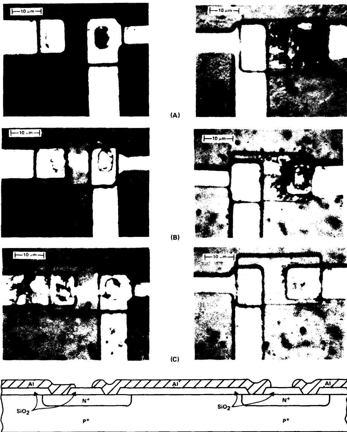
Figure 21. Contacts of HCSO1 Test Structures with (A) Al, (B) Al+Cu and (C) Al+Cu+Si Films Tested at 195°C Under a Current Stress of 1 \times 10^6 A/cm 2 .
