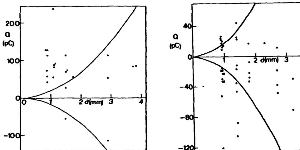
**Figure 1.** Charge-size ( $Q/d$ ) coincidences measured in the 65 seconds of successive penetrations on 15 August 1977. The solid lines are theoretical maxima for the inductive mechanism operating in a breakdown field  $\pm 300 \text{ kVm}^{-1}$ . The numbers attached to certain points are the numbers of observations at those points.
