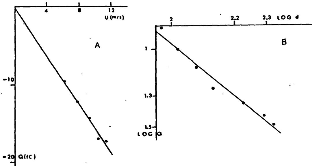
Figure III.1 The charge transferred to a hailstone at  $-10^{\circ}\text{C}$  by a small ice sphere, (A) as a function of velocity,  $U$ , for a  $100\mu\text{m}$  sphere, (B) as a function of sphere size,  $d$ , ( $U = 8\text{ ms}^{-1}$ )
