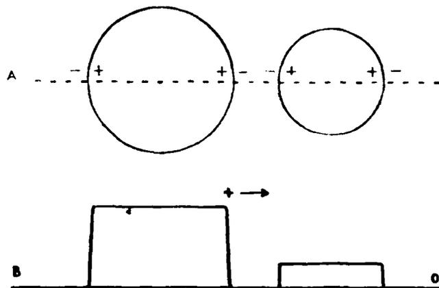
III.6 A. Differing dipole layers on the surface of two uncharged ice spheres. B. The potential variation along the dotted line in Figure A. The arrow shows the direction of charge flow when the spheres touch.
