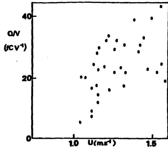
Figure II.4: The measured variation of  $Q/V$  with impact parameter  $U$ .  $10^{-4}\text{M NaCl}$ ;  $T=-12^\circ\text{C}$ .
