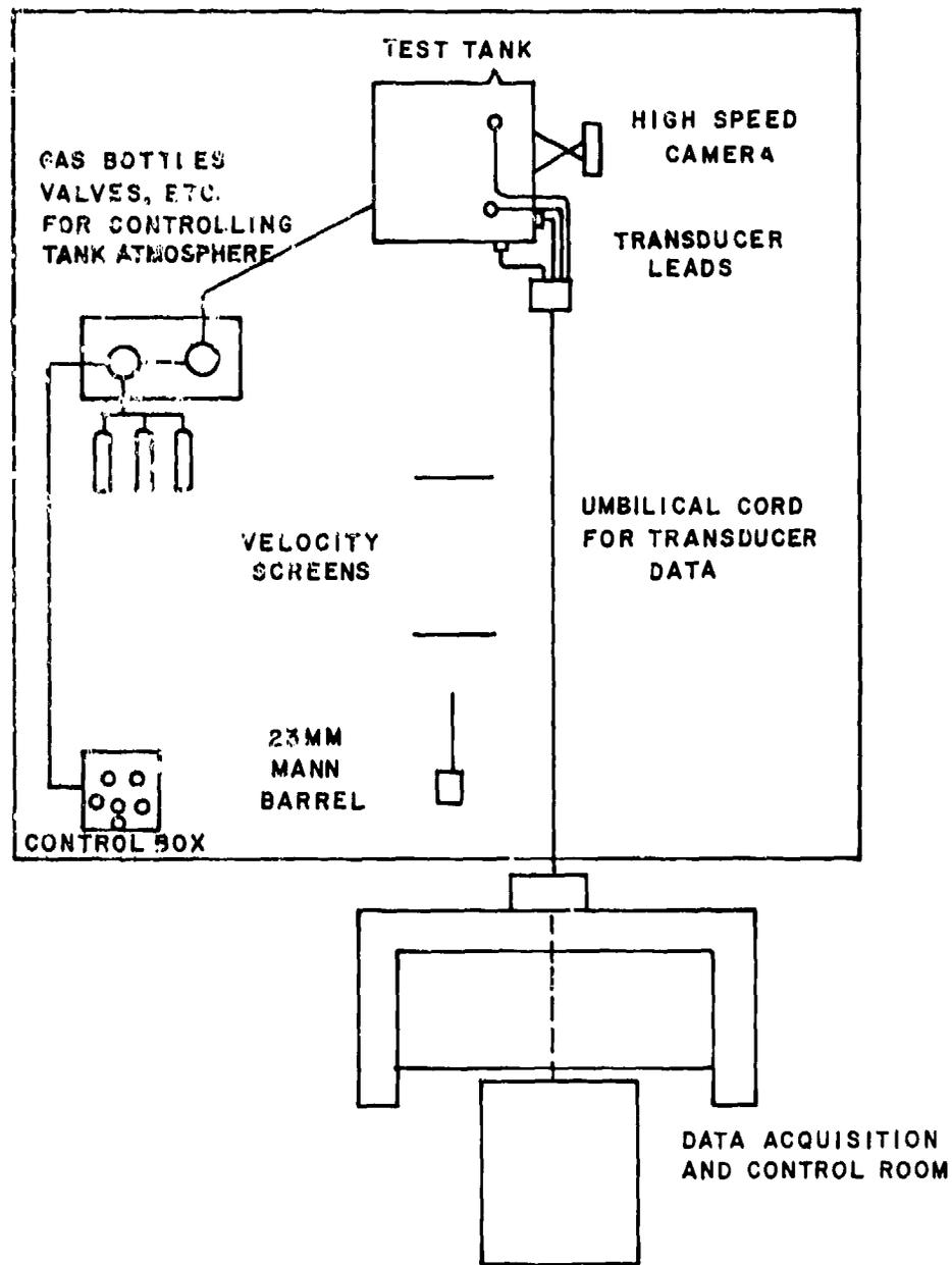
Figure 15. Ballistic Test Site and Equipment
