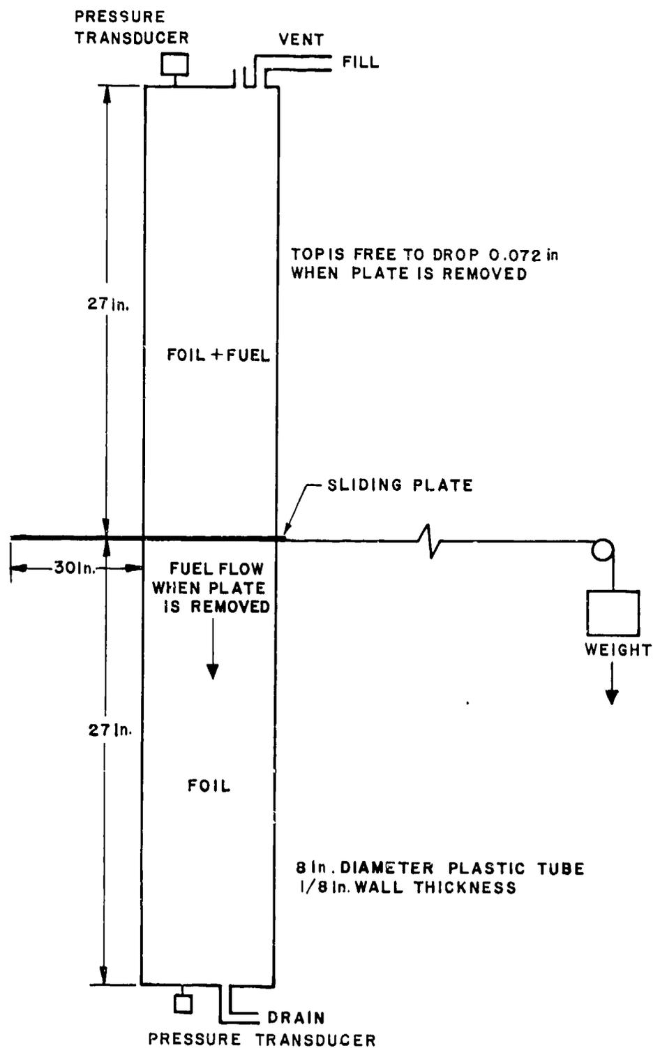
Figure 36. Test Set-Up for Fuel Drop Tests
