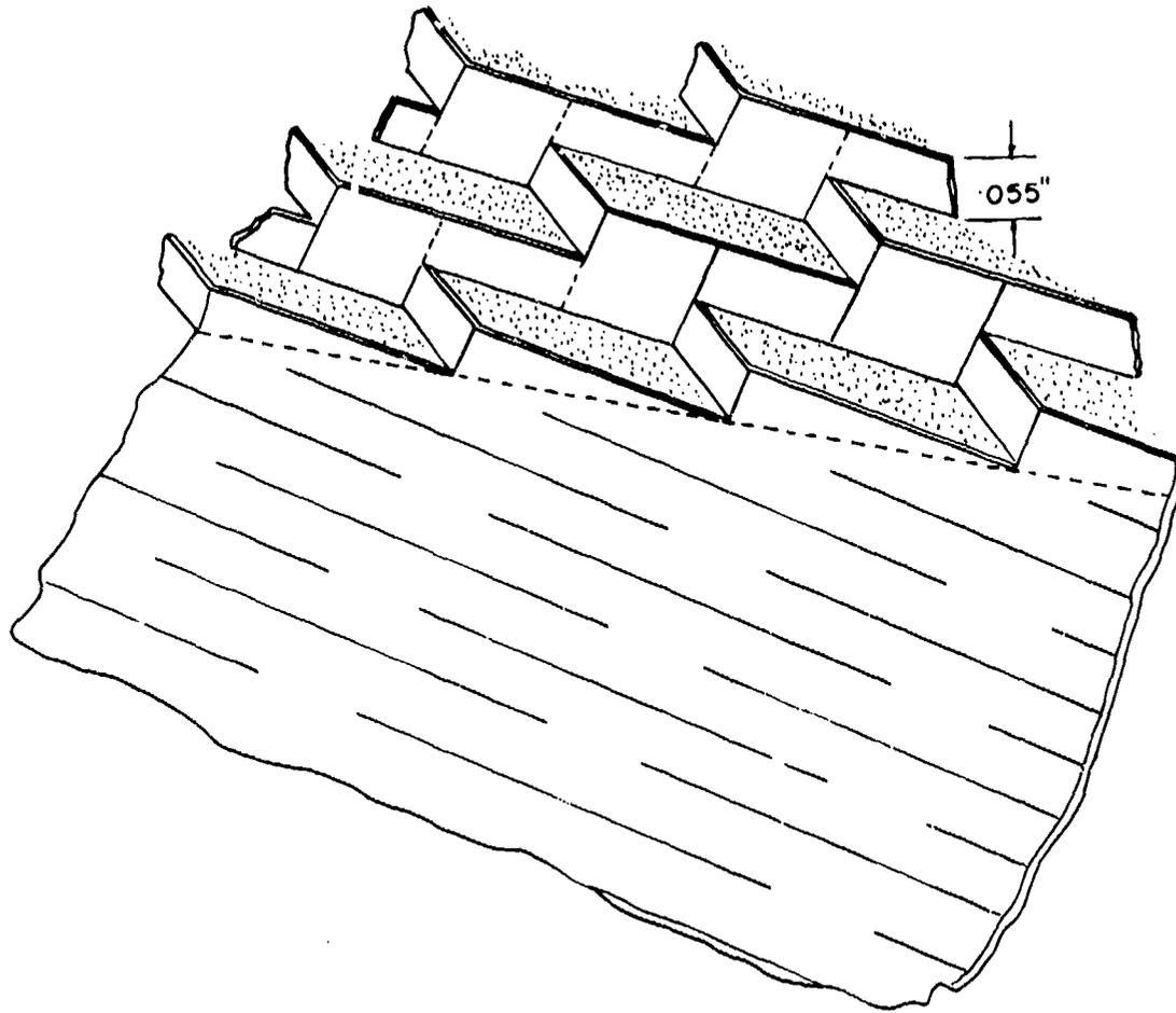
Figure 1. Transition from Slit to Expanded Foil
