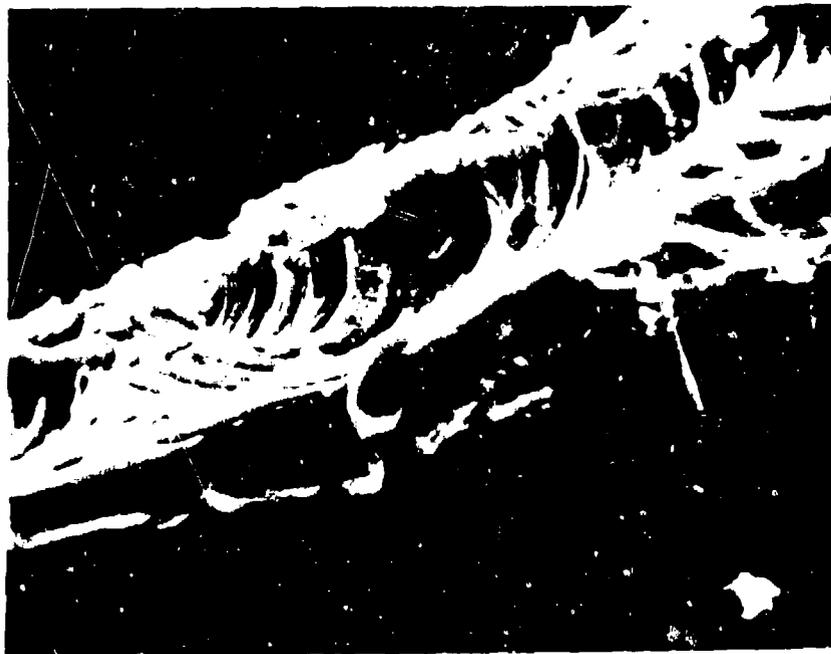
Figure 29. Slit Edge of Aluminum Foil Cut by Guillotine
