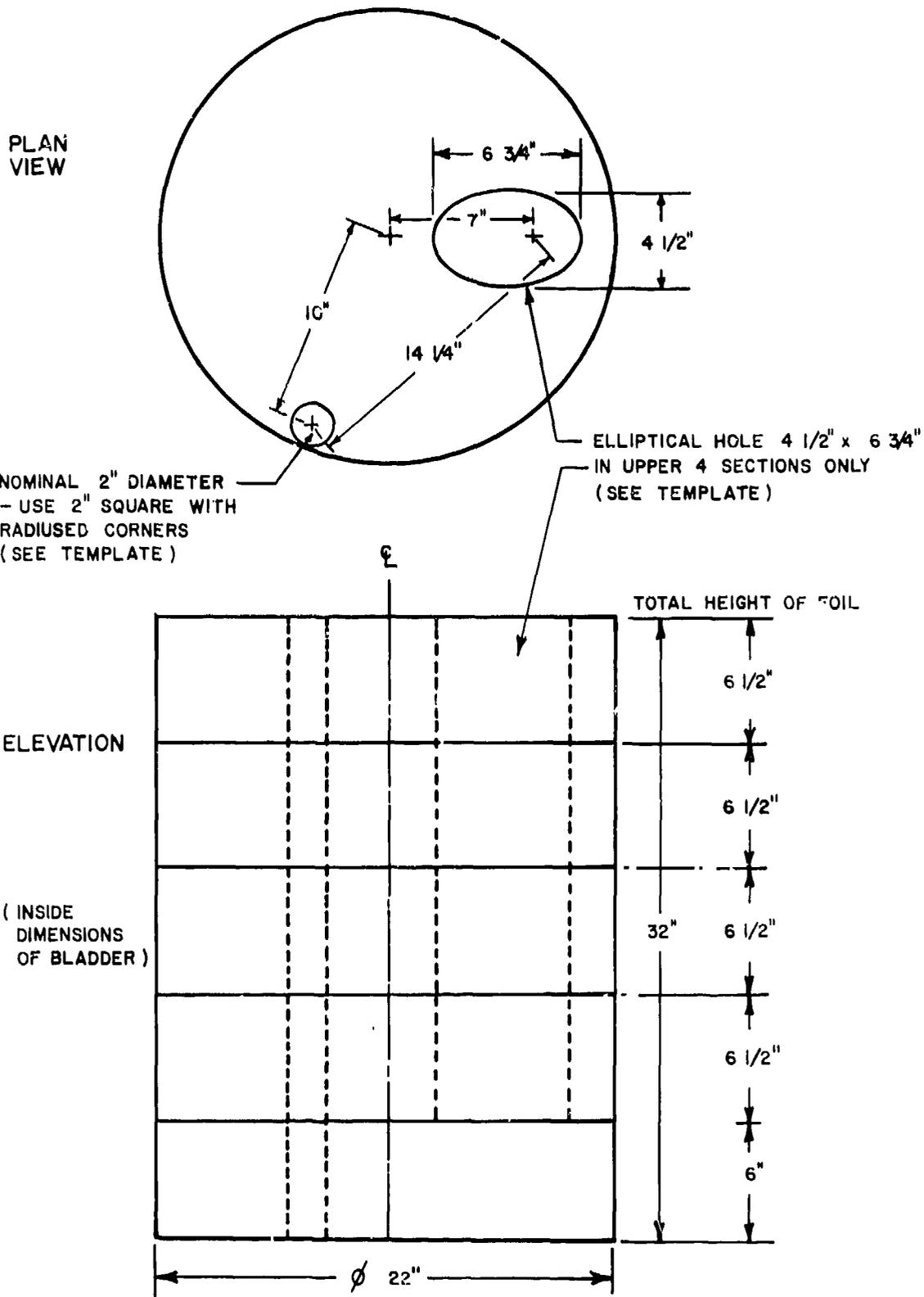
Figure 52. Detail Drawing of Explosafe Drum Installation
