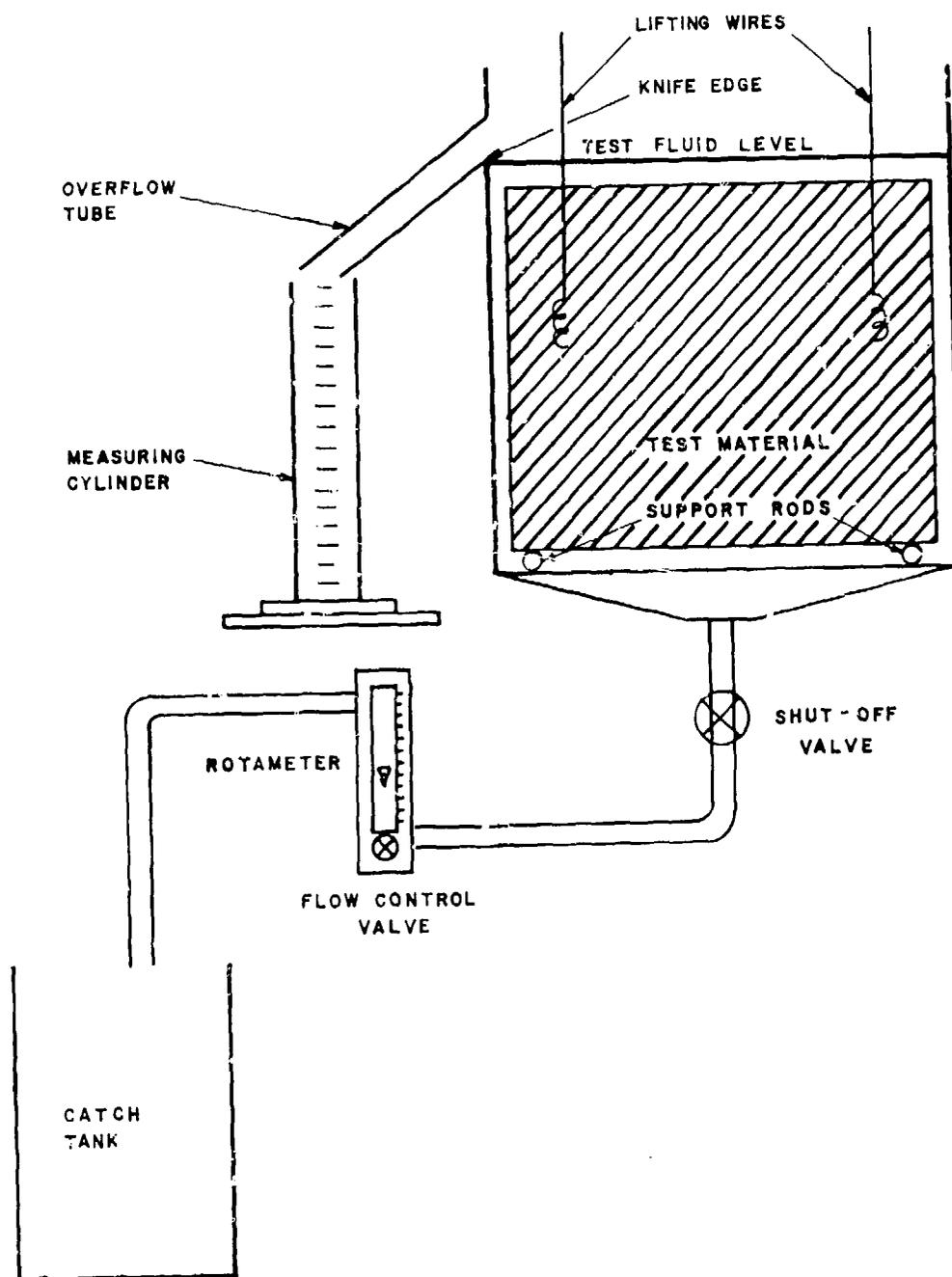
Figure 30. Retention and Displacement Test Rig
