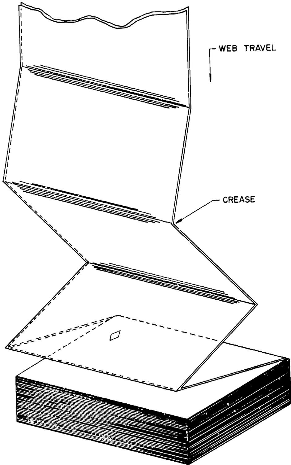
Figure 3. Fanfolding Expanded Foil into Rectangular Batt
