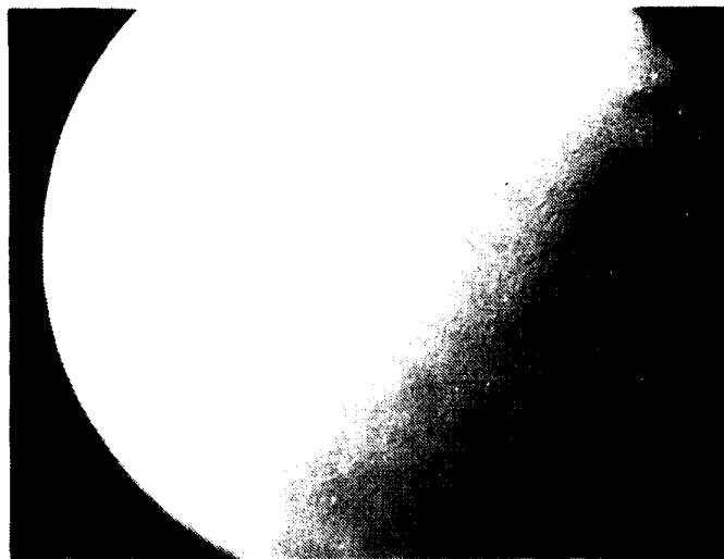
Figure 24. Nomarski interference contrast micrograph of sample L16; 1.2 \text{ J/cm}^2 double-frequency laser irradiated.
