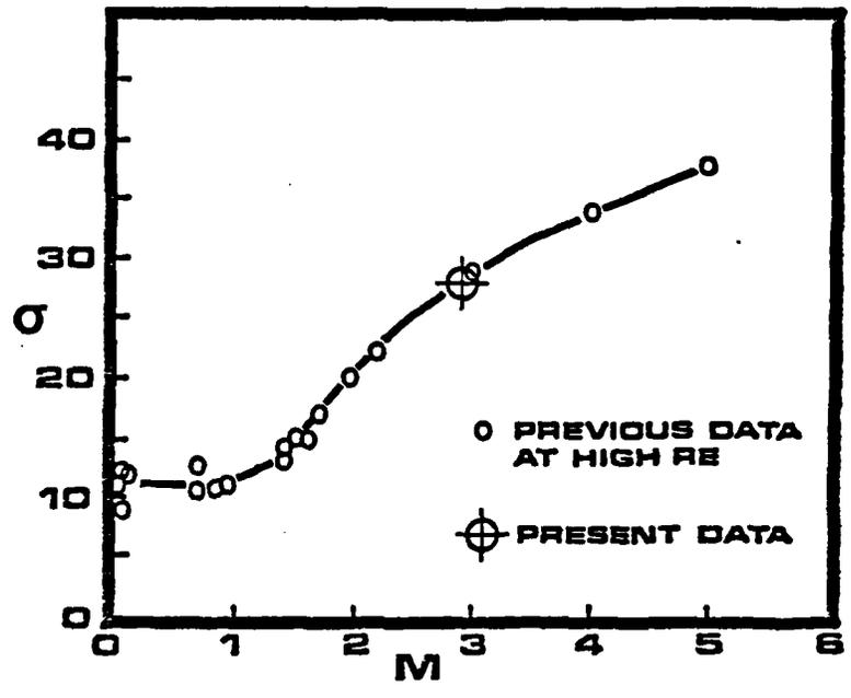
Figure 9 - Variation of Shear Layer Spreading Parameter, Sigma, vs. Mach Number.
