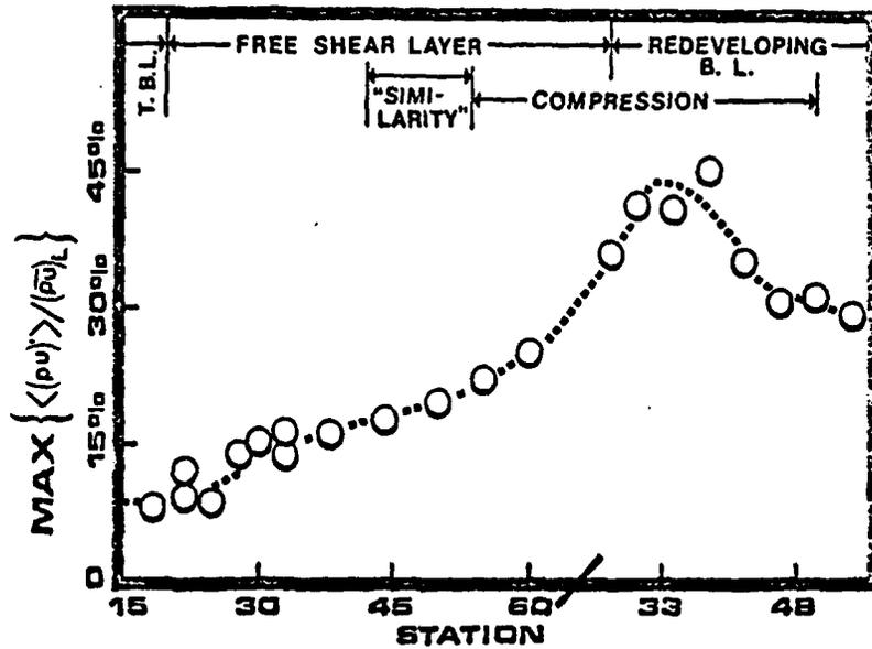
Figure 13 - Plot of Local Maximum RMS Mass Flow Fluctuations vs. Distance Along the Entire Length of the Interaction.
