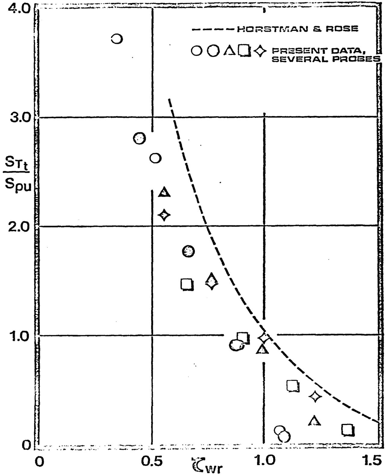
Figure 20 - Plot of Hot-Wire Sensitivity Coefficient Ratio vs. Overheat Ratio.
