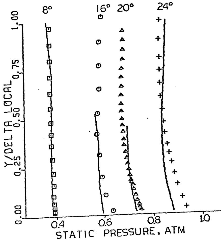
Figure 4 - Comparison of Experimental and Computed Downstream Static Pressure Profiles for the Four Compression Corner Flowfields. (Profile Locations are at  $x/\delta_0 = 5$  for  $\alpha = 8, 16,$  and  $24$  deg and  $x/\delta_0 = 2.75$  for  $\alpha = 20$  deg.)
