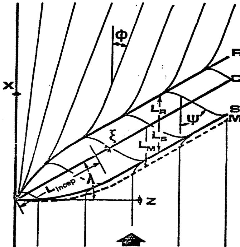
Figure 15 - General Sketch of Surface Flow Pattern on Swept Compression Corner with Definition of Parameters.
