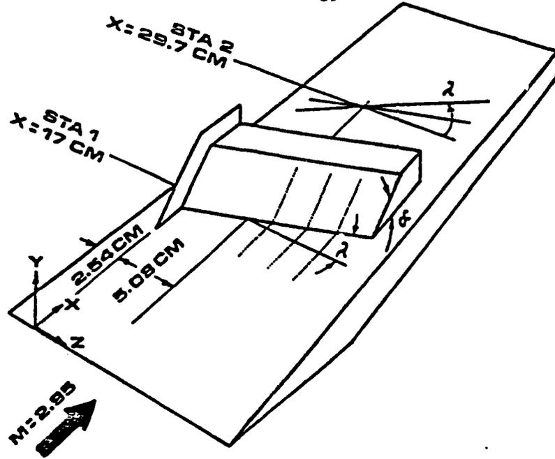
Figure 14 - Sketch of Experimental Configuration
