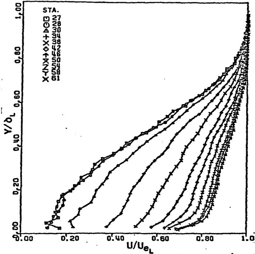
Figure 12 - The Redevelopment of Normalized Mean Velocity Profiles in the Boundary Layer Downstream of Reattachment.
