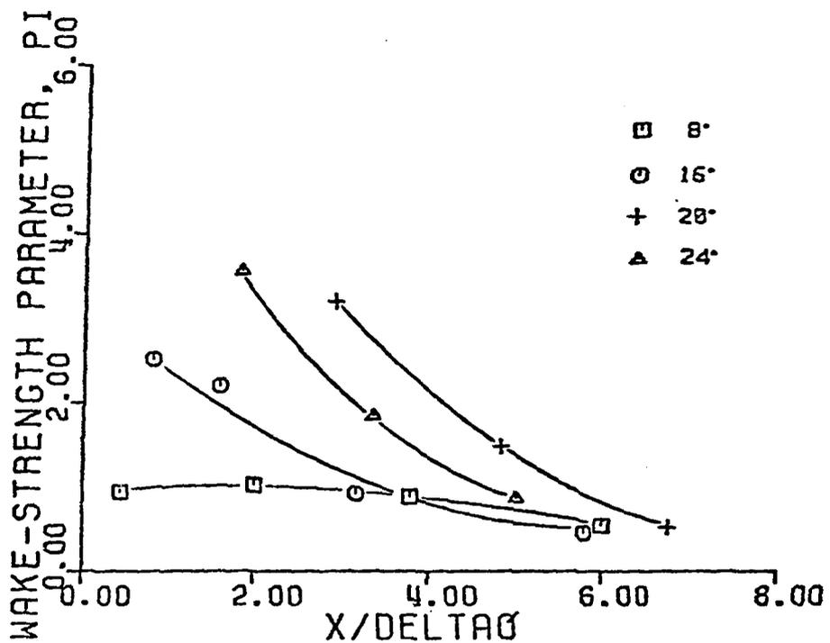
Figure 3 - Decay of the Velocity Profile Wake-Strength Parameter with Distance Downstream of Each Compression Corner.
