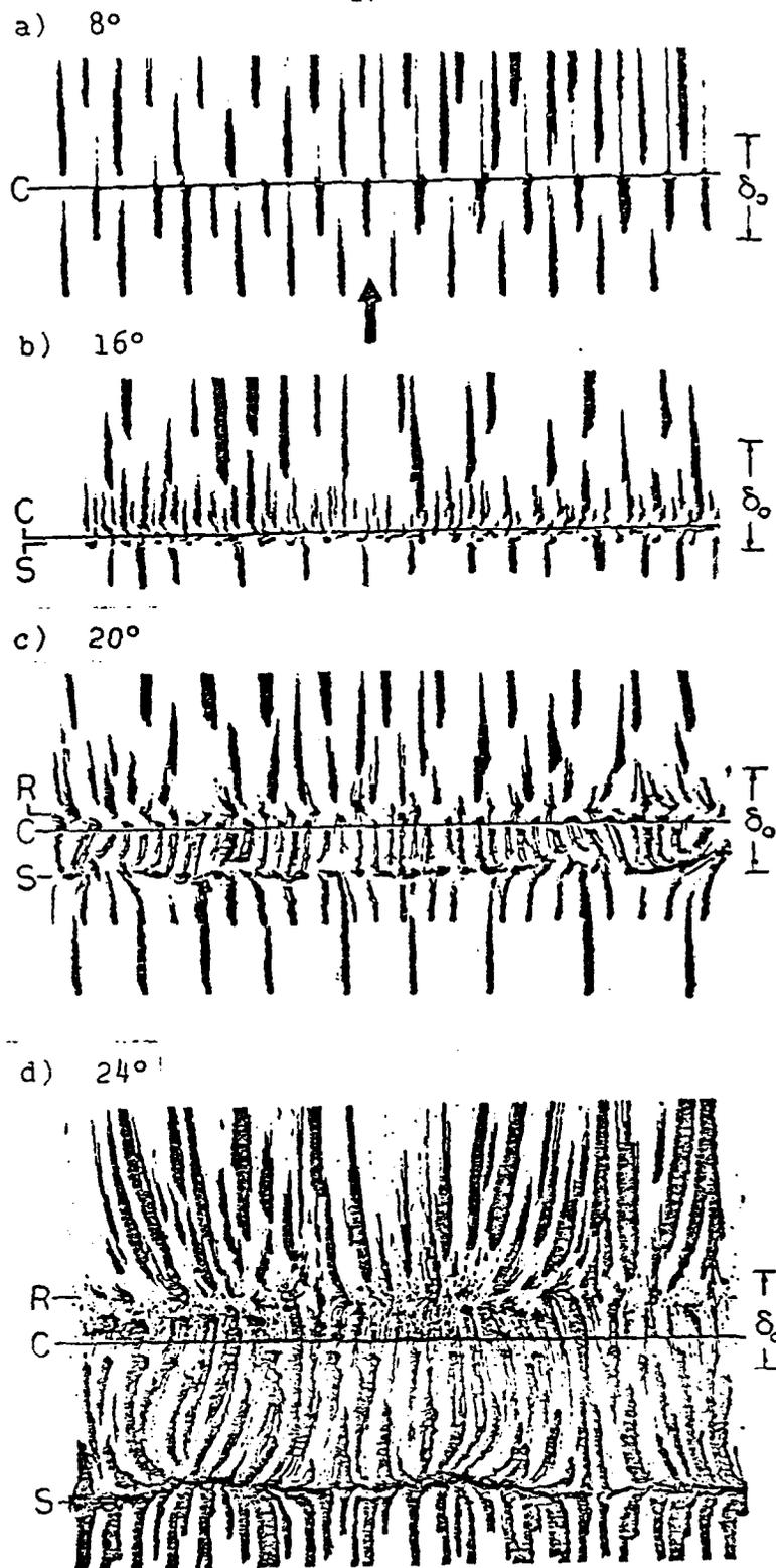
Figure 2a-d - Surface Streak Patterns From the  $8^\circ$ ,  $16^\circ$ ,  $20^\circ$ , and  $24^\circ$  Compression Corner Flowfields. (S,C, and R Denote Separation, Corner, and Reattachment Locations, Respectively. The Streamwise Direction is From Bottom to Top in Each Case. The Incoming Boundary Layer Thickness,  $\delta_0$ , is noted for a Scaling Reference.
