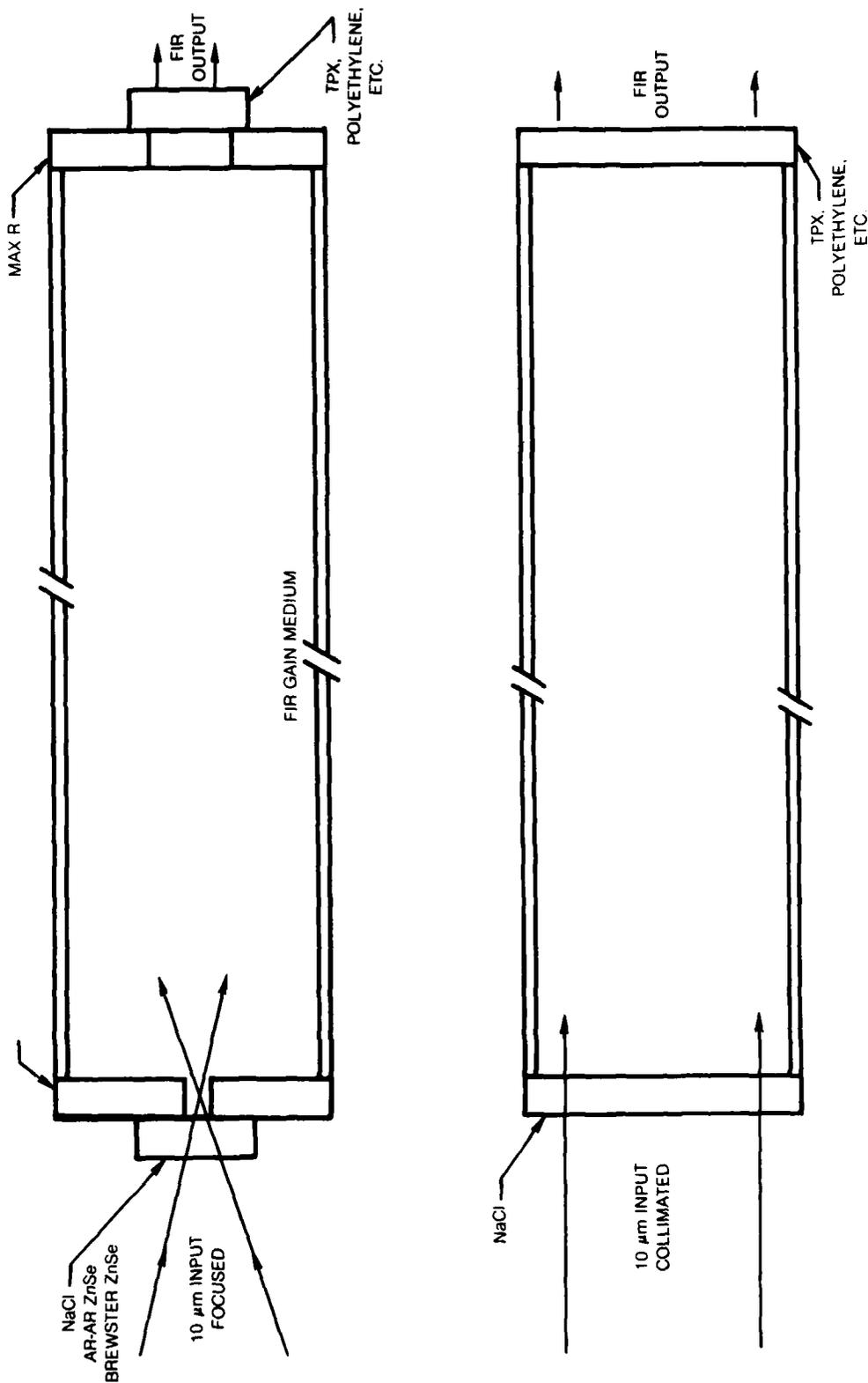
**ONE METER STEEL FIR GAIN CELL**
