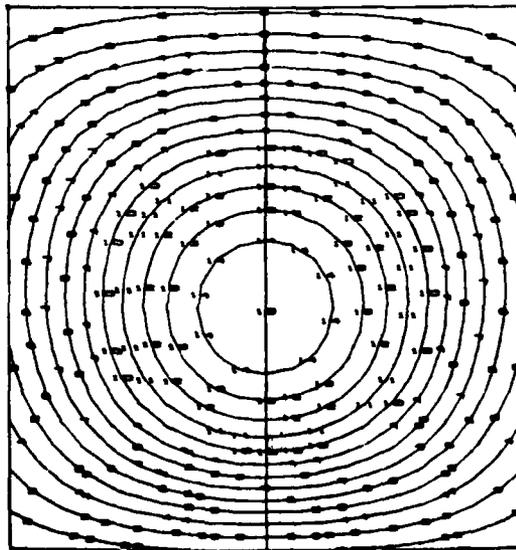
Figure 6. Computer Generated Displacement Plot for Center Windshield Under 1 PSI Loading.
