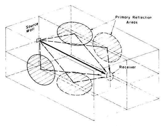
FIGURE 6. Three-Dimensional View of Chamber Primary Reflection Areas.
