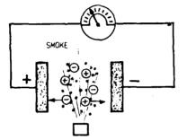
FIGURE 12. Ionization Smoke Detector.
