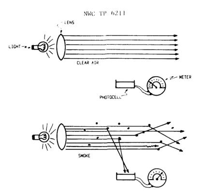
FIGURE 13. Side-Scattering Photoelectric Smoke Detector.
