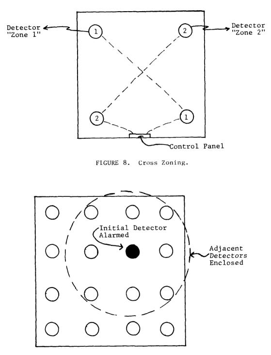
FIGURE 9. Priority Matrix: Overall Alarm Activation by Alarm of Detector Adjacent to Initial Alarming Detector.
