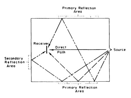
FIGURE 5. Reflections in Anechoic Chamber.
