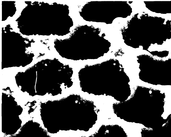
Figure 34. Example of Major Damage to LVFE Structure (Cathode L19D-B, Test HP-21) at 13 Torr, X7500, 45°.
