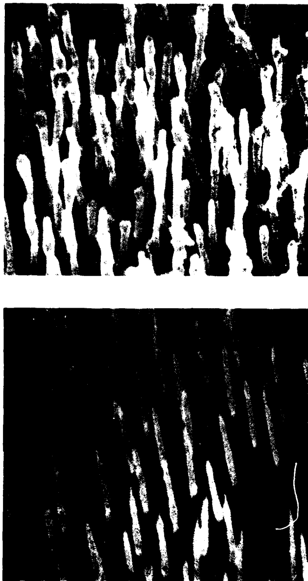
Figure 40. Examples of Pre-test Exposed Pin Composite Electrodes, (a) Gd_2O_3-Ce_2O_3-Mo , (b) UO_2-W , X5000, 45^\circ .
