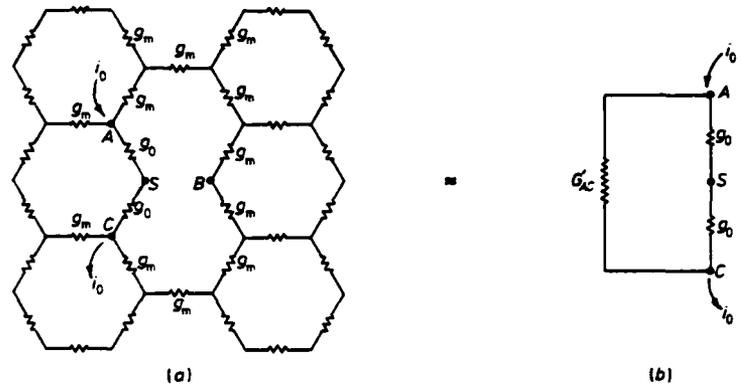
Figure 1. Single site  $S$  of a honeycomb lattice for the calculation of the longitudinal conductivity. The cluster of three conductances  $g_0$  around  $S$  are located within an effective network of conductances  $g_m$ . From symmetry the conductance  $g_{SB}$  can be ignored.
