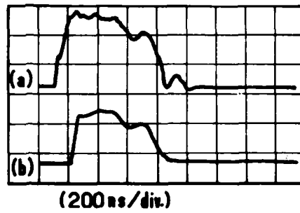
Fig. 2 Electron beam current (a) and laser (b) waveforms. The peak current corresponds to a e-beam of 10 \text{ A cm}^{-2} in laser cavity. Gas Ne/Xe/HCl; T=120\text{K} T_{\text{mirror}}=0.1\% and 5\% .
