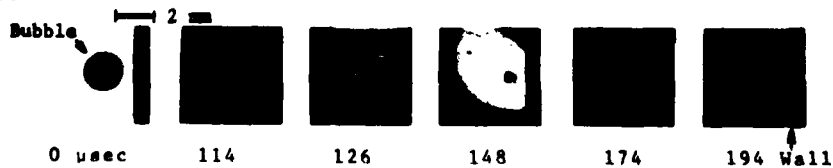
Fig.10 Microjet formation from the bubble in the neighbourhood of the solid boundary
