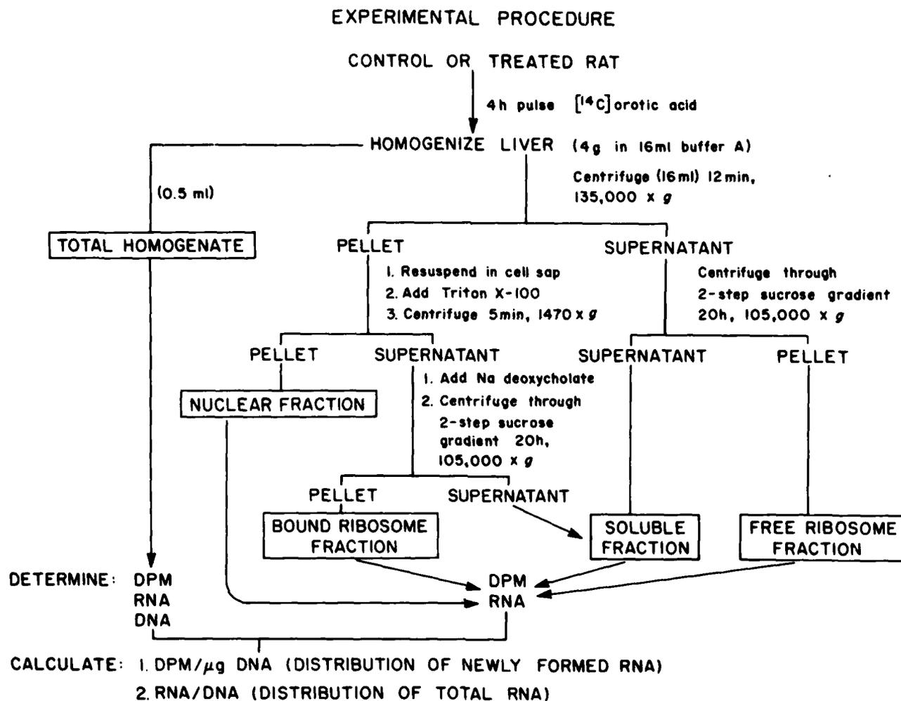
FIG. 1. Procedure for subfractionation of rat liver and determinations and calculations performed on each fraction.
