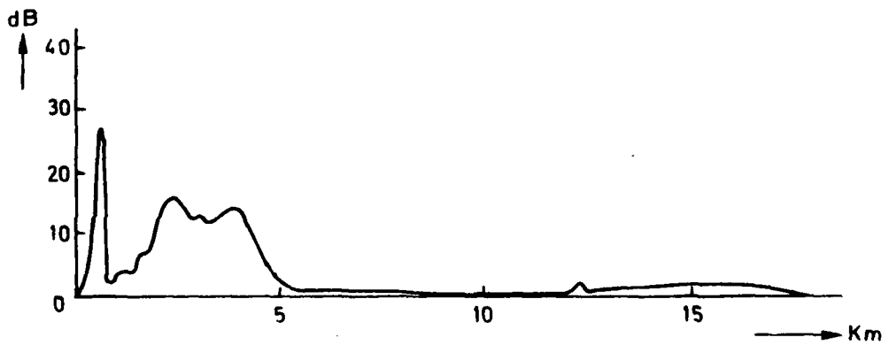
Figure 2 Raw radar data sample recorded August 2, 1979, 11.08 GMT. Horizontal scale slant range; vertical echo intensity in dB.
