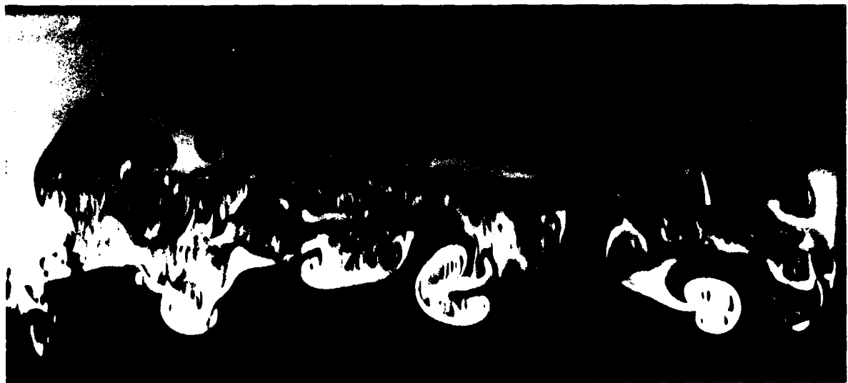
Fig. 3 Cross sectional views normal to flow direction of mixing layer in water. U_1 \doteq 32 cm/sec, U_2 \doteq 11 cm/sec, x = 15 cm. a) Section between primary vortices b) Section through a primary vortex
