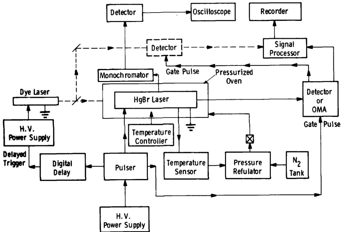
Figure 3. Spectroscopic apparatus designed to measure the fluorescence, absorption and gain features of pulsed TlHg discharges.
