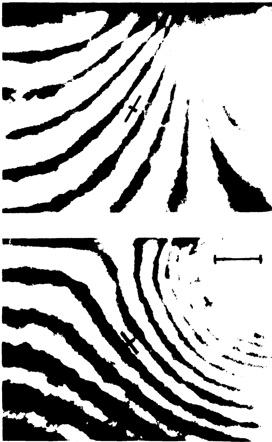
Fig. 1 — Complementary interferograms of a laser-produced plasma taken simultaneously with a folding-wave-front shearing interferometer. The axis of symmetry is at the bottom in both cases and a 200 micron marker is given. Note how, in the normal interferogram on the left, the fringes bend away from the center while, in the inverted interferogram on the right, they bend toward the center.
