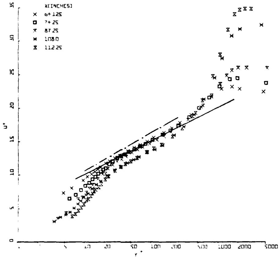
Figure 20. Mean velocity profiles of unsteady flow A in  $U^+$  vs.  $\log y^+$  coordinates.
