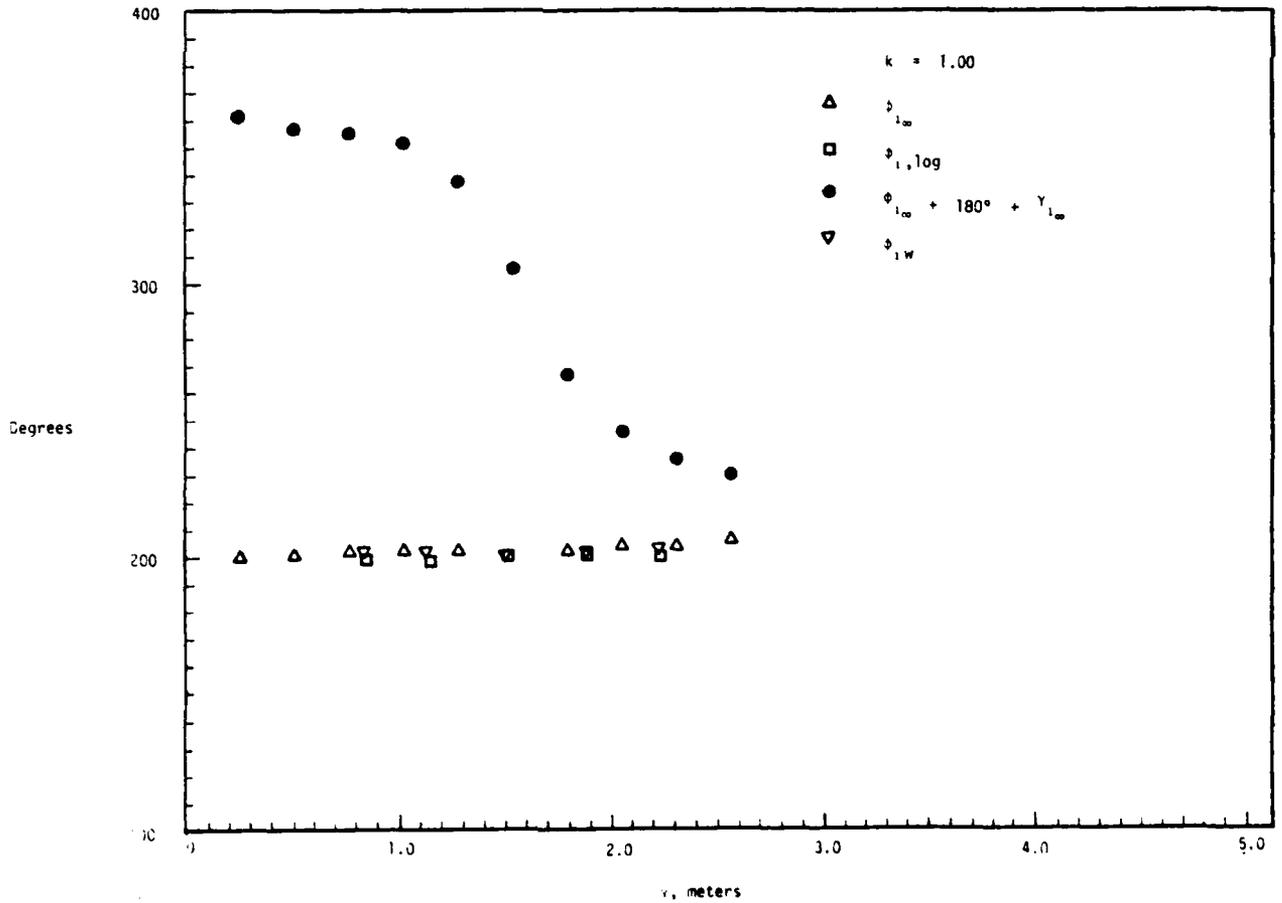
Figure 5. Phase angles of first harmonics for  $k = 1.00$  flow:  $\phi_{1,\infty}$ , free-stream velocity;  $\phi_{1,\log}$ , logarithmic region velocity; pressure gradient,  $\phi_{1,\infty} + 180^\circ + \gamma_{1,\infty}$ ; wall shearing stress  $\phi_{1,w}$ .
