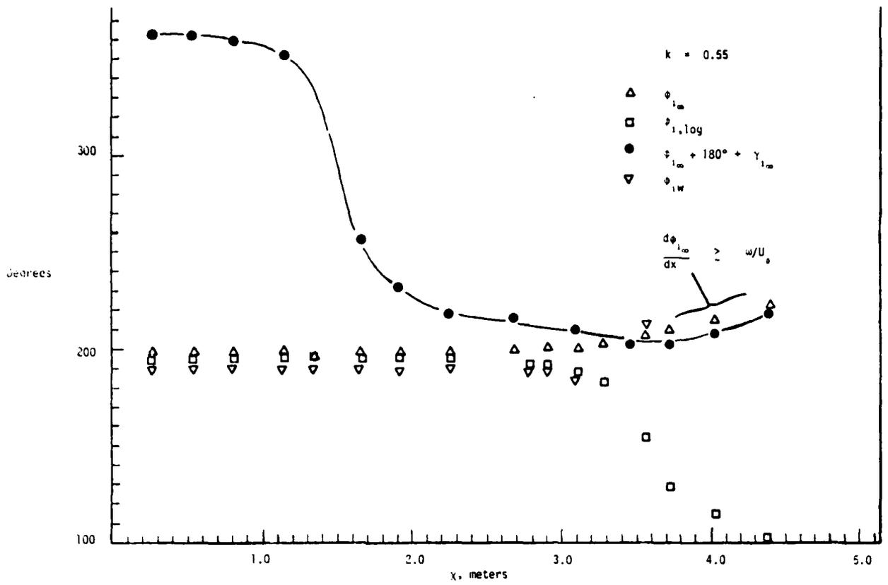
Figure 4. Phase angles of first harmonics for  $k = 0.55$  flow:  $\phi_{1,\infty}$ , free-stream velocity;  $\phi_{1,\log}$ , logarithmic region velocity; pressure gradient,  $\phi_{1,\infty} + 180^\circ + \gamma_{1,\infty}$ ; wall shearing stress  $\phi_{1,w}$ .
