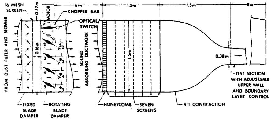
Figure 1. Schematic of the SMU Wind Tunnel
