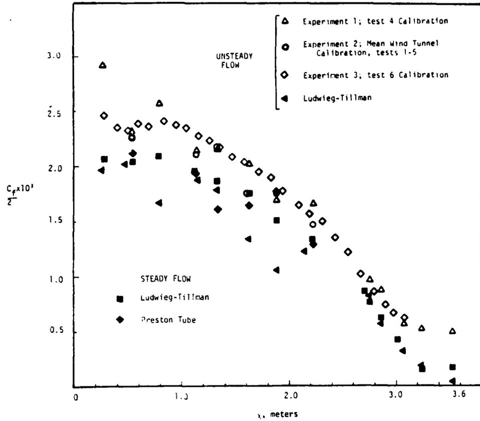
Figure 18. Time-averaged surface shearing stress for  $k = 0.55$  unsteady flow and for steady flow with same freestream mean velocity distribution.
