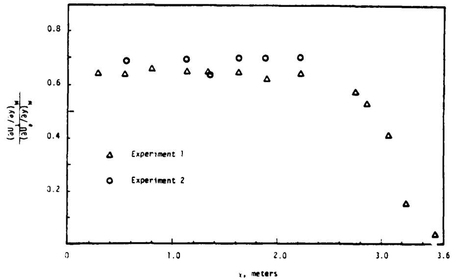
Figure 19. Amplitude of first harmonic to mean wall shearing stress,  $k = 0.55$  flow.
