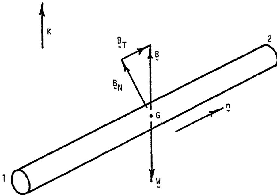
Figure 5. Weight and Buoyancy Forces Acting on the Cable Segment
