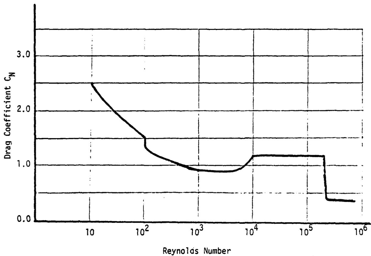
Figure 4. Normal Drag Coefficient (References [47-54]).
