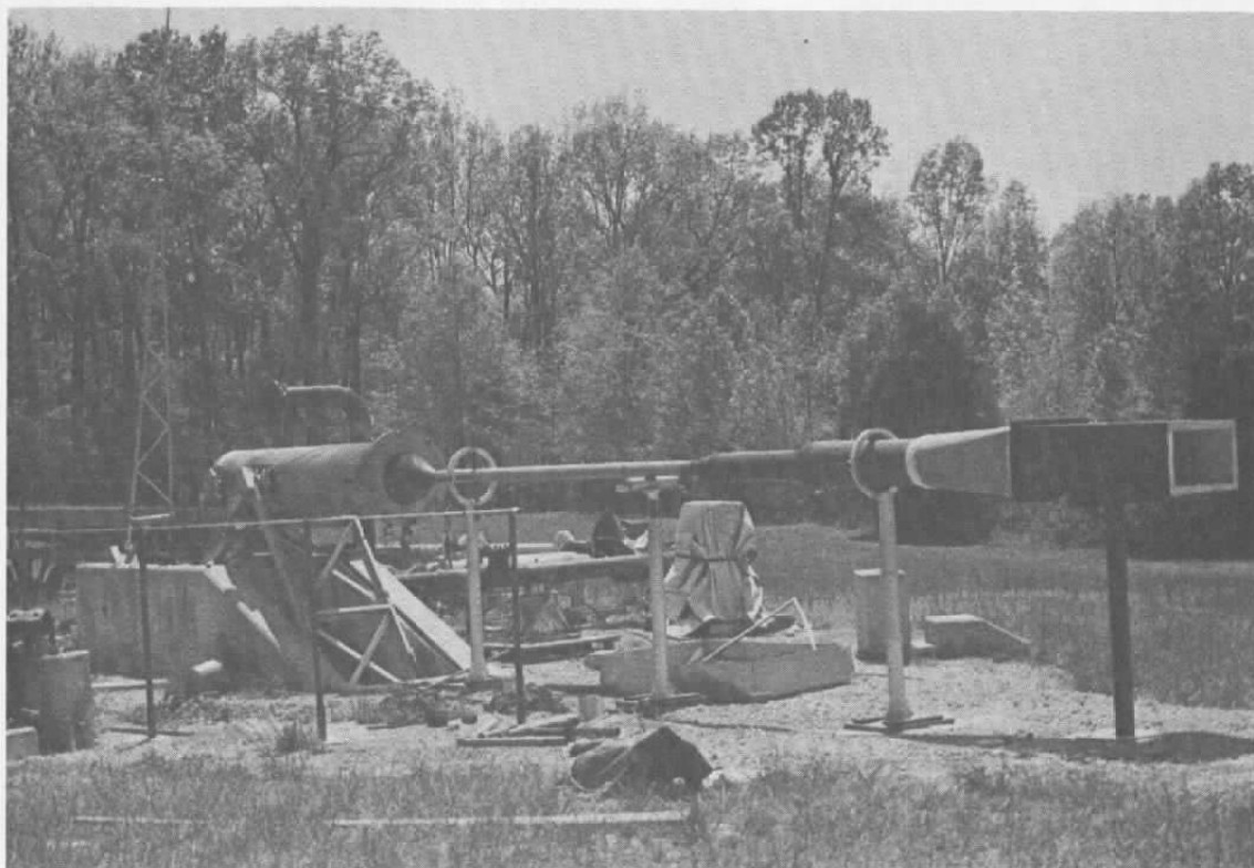
Fig. 5. Exhaust Duct with Liner.
