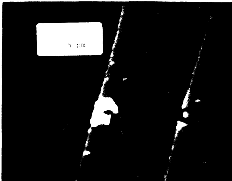
Figure 22. Low-voltage SEM of aluminum line passivated with SINCAP after corrosion at 85°C and 85% rh. Line at left was the cathode.
