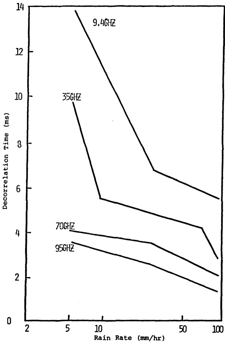
Figure 4. Decorrelation time of radar backscatter from rain.
