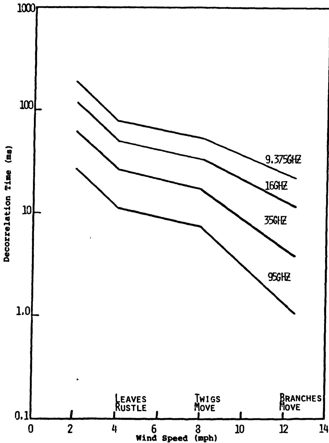
Figure 2 Decorrelation time of radar backscatter from trees
